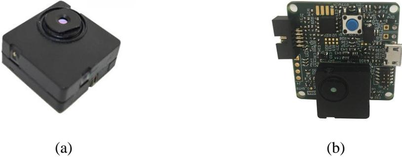
Figure 6-2: The pictures of LWIR Camera Core (a) and evaluation board with LWIR Camera Core connected (b).
