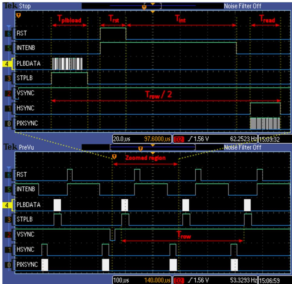
Figure 4-4: The test results of some of the important digital signals generated by the digital controller.
