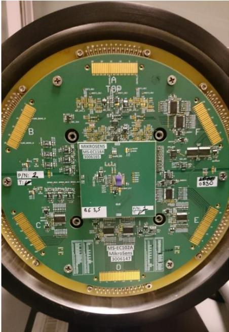
Figure 4-1: Dewar motherboard and proximity card with wire-bonded sensor.
