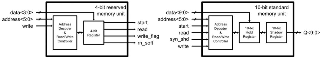
Figure 3-16: Block diagram of 10-bit memory unit.
