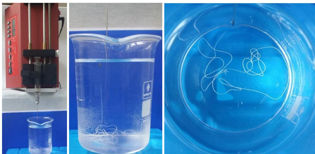
Figure 2.1. Wet spinning setup. Spinning of fiber (a) overall view, (b) zoomed side view and (c) zoomed top view.
