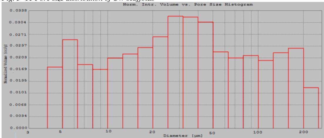
Fig. 3- 12 Pore size distribution of CW scaffolds
