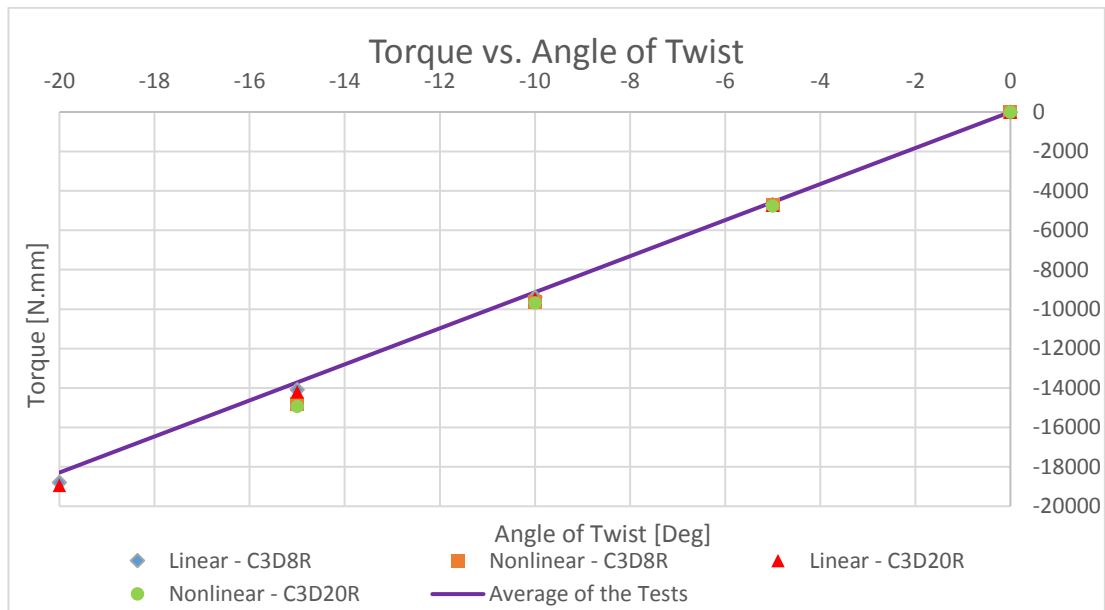
Figure 5.7: Torque - Angle of Twist Curves Obtained from the Tests and FEA for the Beams with Tabs
