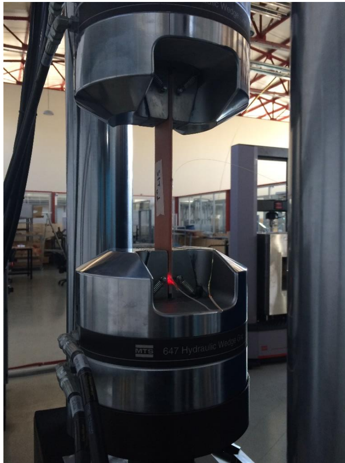
Figure 4.26: Fiber Optic Cable Breakage between the Grips (S1TTUD)
