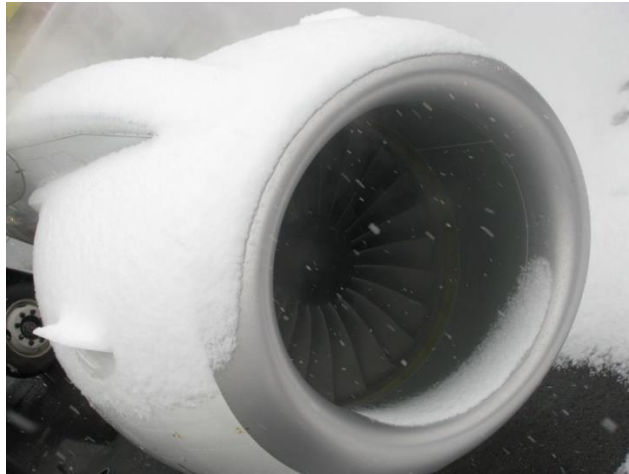
Figure 1: An example of ice accumulation on an engine nacelle [13]
