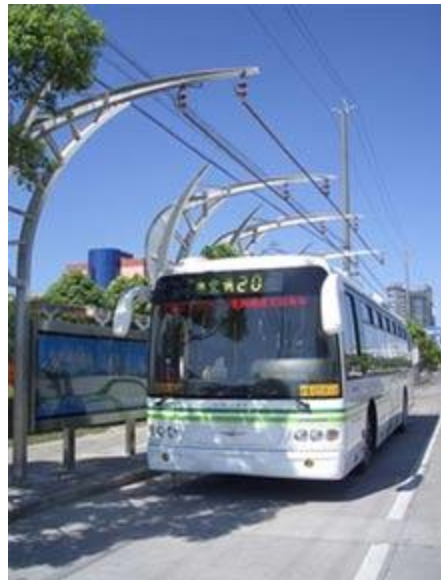
Figure 1.2 A photo of an electric bus that operate only with supercapacitors in Shanghai, China [11].
