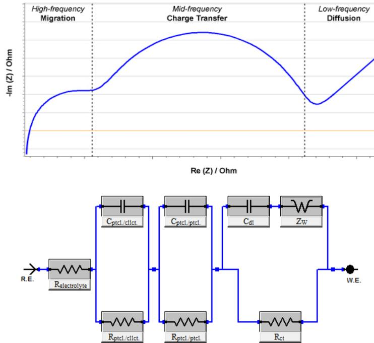
**Figure 2.2** Representative EIS pattern for a negative electrode material of NiMH battery and corresponding equivalent circuit.
