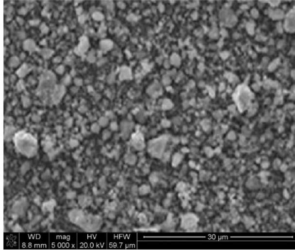
*Figure 3.4 SEM image of the 20 hours milled powders.*
