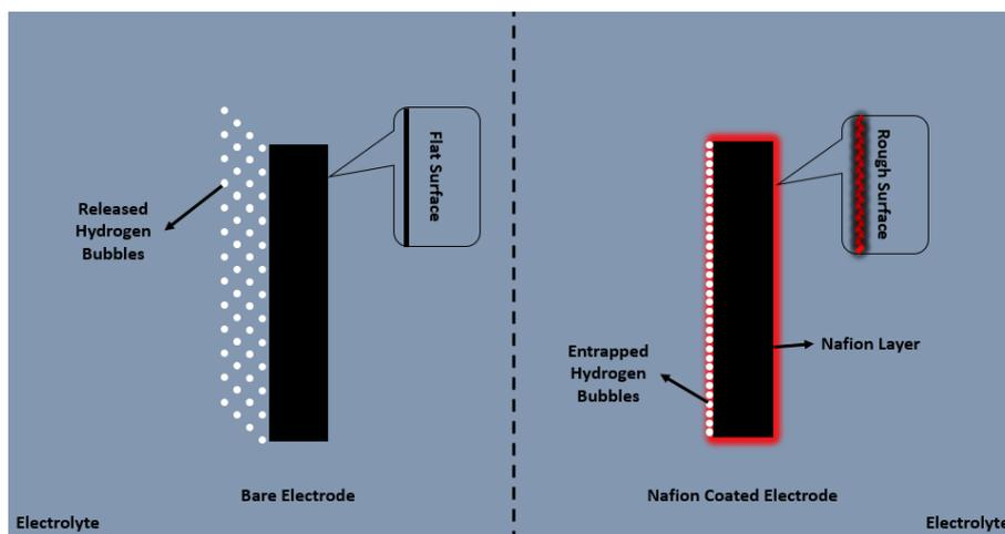
**Figure 5.1** Hydrogen bubble formation and disintegration at the electrode. Left side image represents the bare electrode and right side shows nafion coated electrode.
