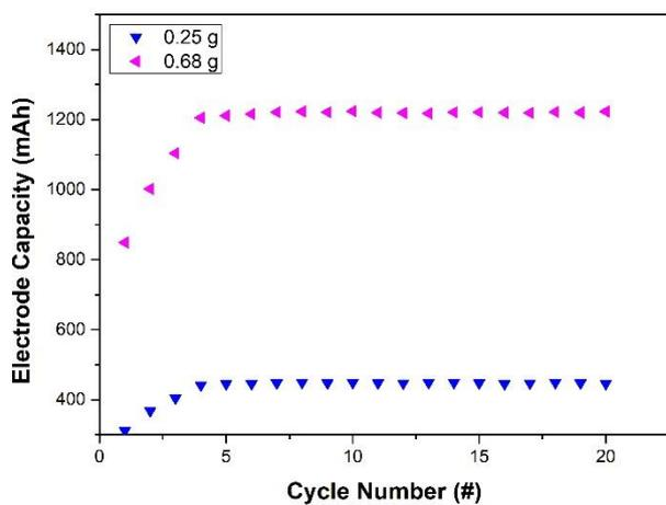
**Figure 4.10** Variation of the electrode capacity with increasing active material. The capacity normalized with respect to mass yields 448 mAh/g with 0.25 g and 451 mAh/g with 0.68 g of active material.
