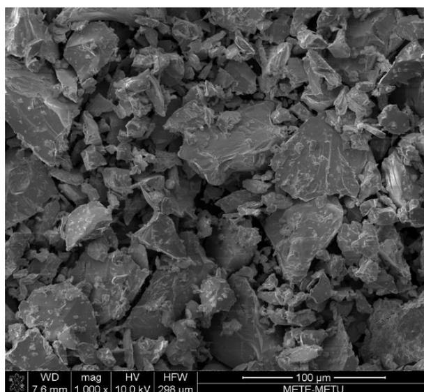
*Figure 4.1 SEM image of A<sub>2</sub>B<sub>7</sub> powder showing the general shape and size of the particles.*
