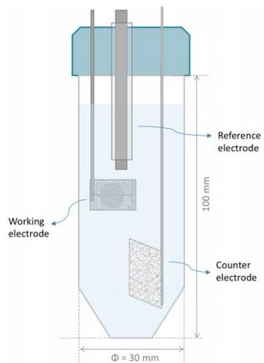
**Figure 3.2** Three electrode cell structure used in the electrochemical tests.
