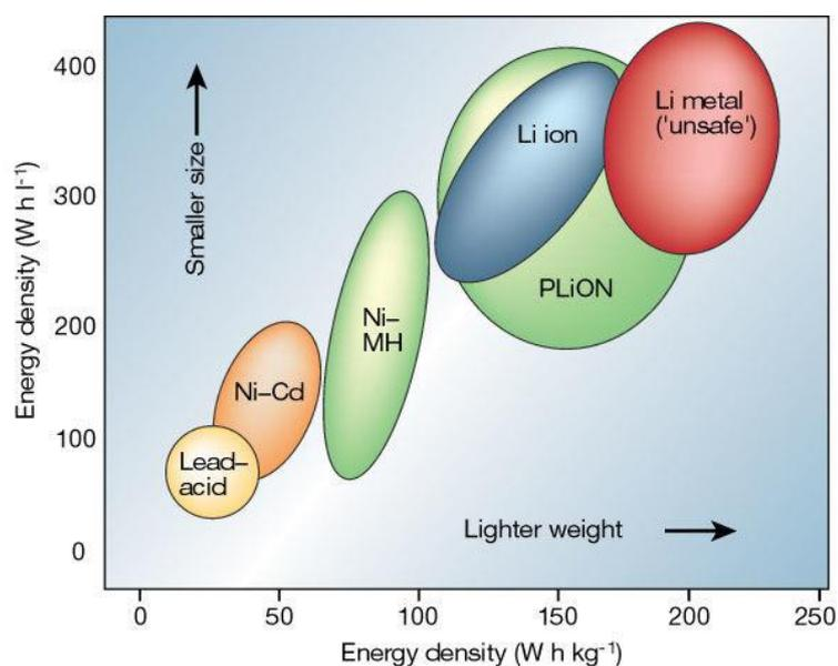
**Figure 1.1** Comparison of the different battery technologies in terms of volumetric and gravimetric energy. Tarascon and Armand (2001).
