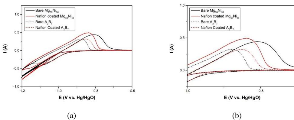
**Figure 4.4** CVs of  $Mg_{50}Ni_{50}$  and  $A_2B_7$  electrodes showing (a) both in bare and nafion coated forms replotted on the same potential vs. current axes and (b) focused window on the anodic potentials.
