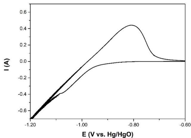
**Figure 3.5** CV of the bare  $Mg_{50}Ni_{50}$  electrode showing the potentials of anodic and cathodic reactions.
