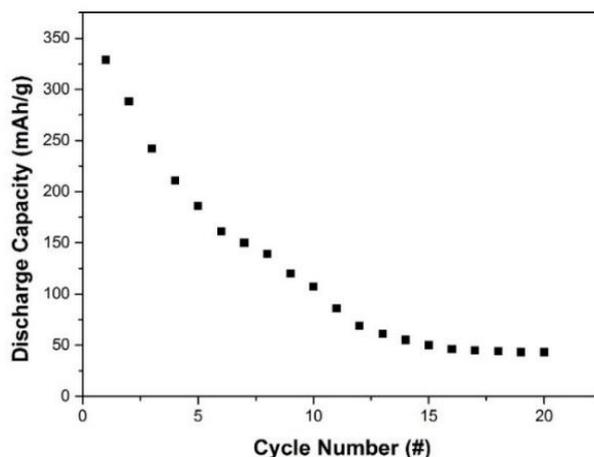
**Figure 3.7** Variation of discharge capacity of bare Mg<sub>50</sub>Ni<sub>50</sub> electrode with cycling.
