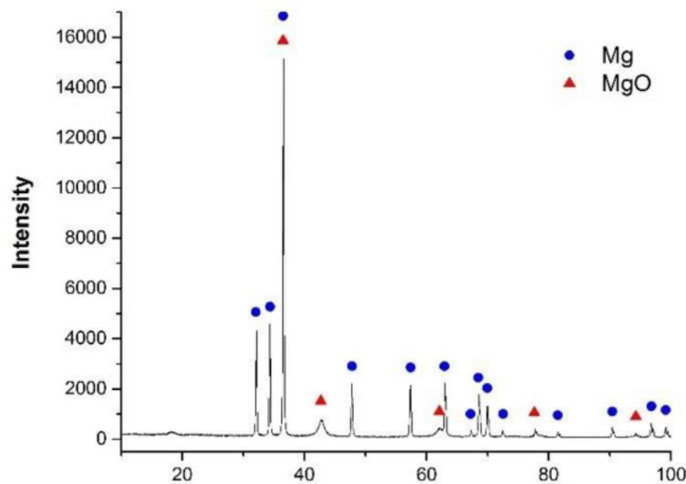
**Figure A.3** XRD spectrum of the encapsulated powders by using citric acid and ethanol. Rietveld analysis conducted on the powders revealed that the amount of MgO formed is 19.1 at. % (Bragg R-factor: 7.8, reduced  $\chi^2$ : 7.8).
