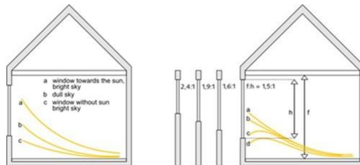
Figure 6. Iso-contour curves of daylight penetration (Frankel and Lyles, 2013)
