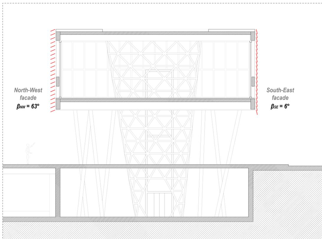
Figure 47. Optimum rotation angle of the panels to achieve the optimum daylight availability of the exhibition space during June.
