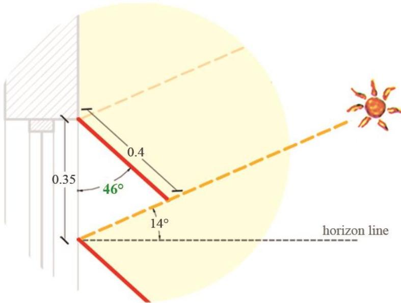
Figure 13. Parametric louvered shading system
