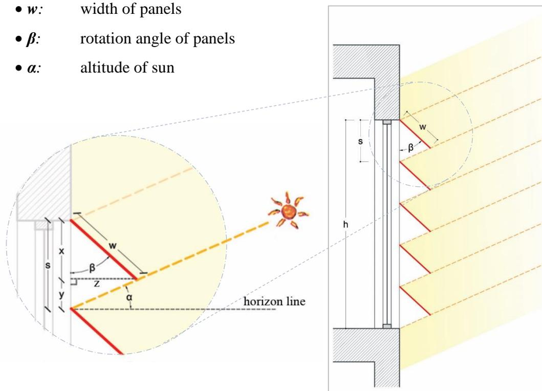
Figure 12. Design parameters of the horizontal louvered shading system
