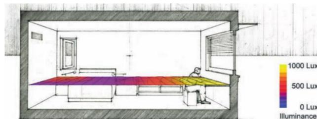
Figure 14. Illumination level on a working plane that is illustrated in false color. The simulation was performed for 2p.m. on March 21 at a workplain with 76 cm height over the floor (Anderson, 2014).
