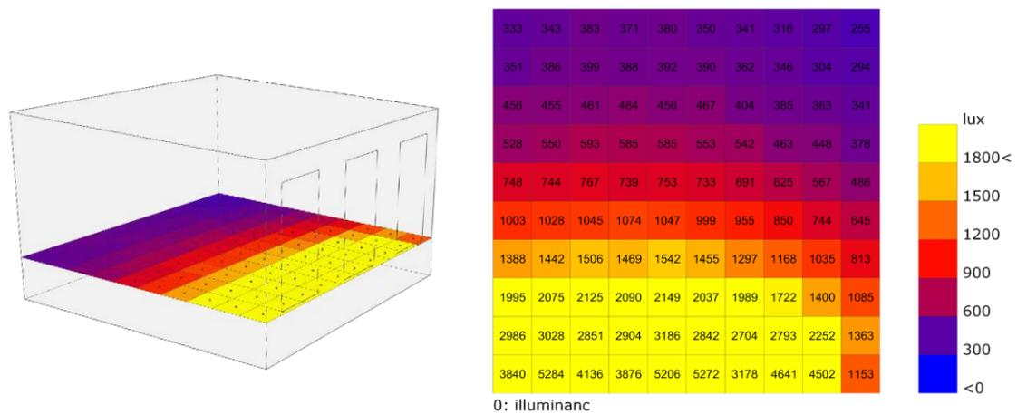
Figure 16. Daylight illumination values (in lux) that are received by grid cells.
