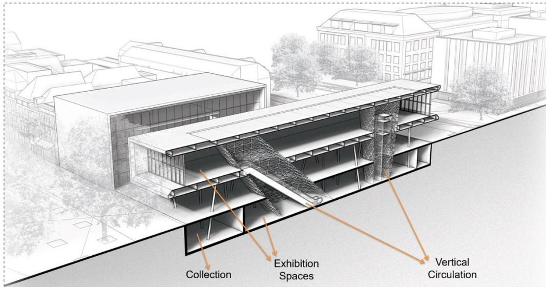
Figure 28. Longitudinal section, demonstrating the vertical circulations within the museum.
