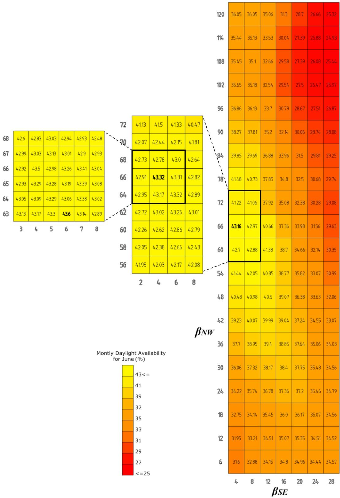
Figure 48. Finding the Optimum Daylight Availability of the exhibition space during June through the parametric design exploration. Developed by the author in Grasshopper.
