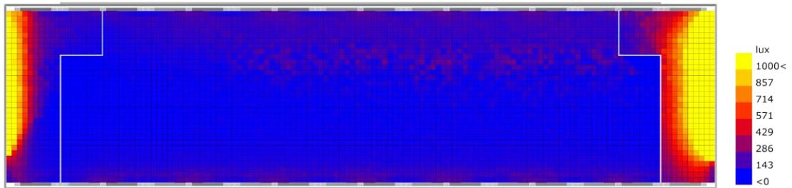
Figure 42. Plan view of the exhibition space illustrating the average level of illumination on the working plane during December at 2 pm.  $\beta$  for South-East and North-West façades were accordingly set as  $8^\circ$  and  $66^\circ$ . Prepared in Honeybee.
