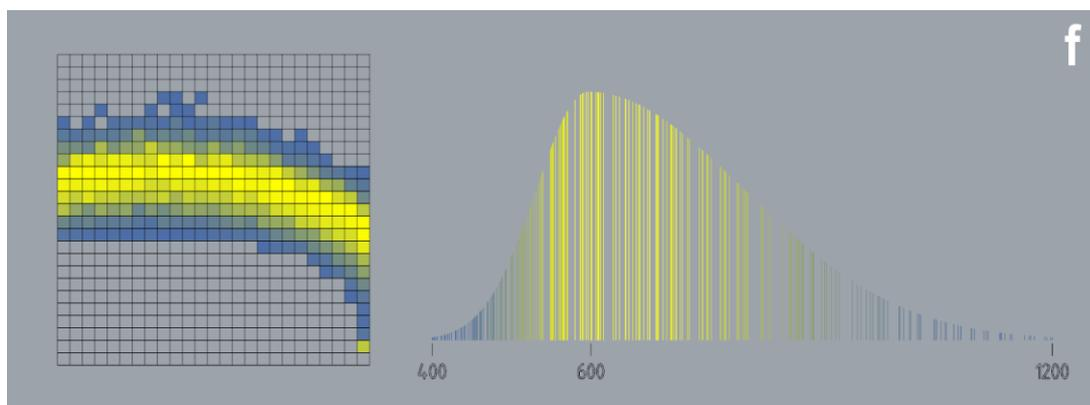
Figure 21. Fuzzy Gaussian membership values, assigned to the range of 400 to 1200 lux in 3 different ways with respect to the desired visual task. Developed by the author in Grasshopper and Honeybee.
