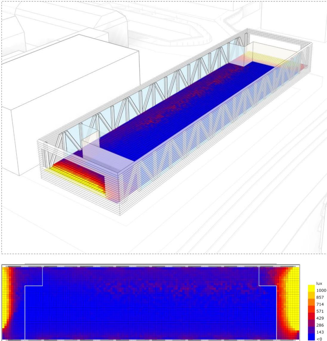
Figure 40: Plan and perspective views of the exhibition illustrating the average level of illumination on the working plane during December at 2 pm.  $\beta$  for South-East and North-West façades were accordingly set as  $8^\circ$  and  $66^\circ$ . Prepared in Honeybee.
