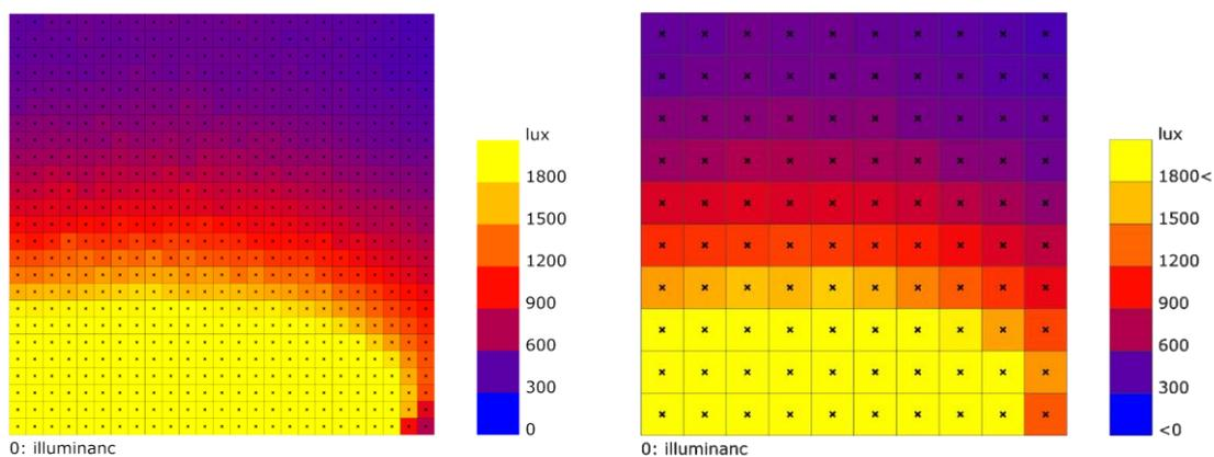
Figure 15. working plane of an instance simulation with different grid sizes. The working plane on the left has a grid size of 20 cm, while the one on the right has a grid size of 50 cm.
