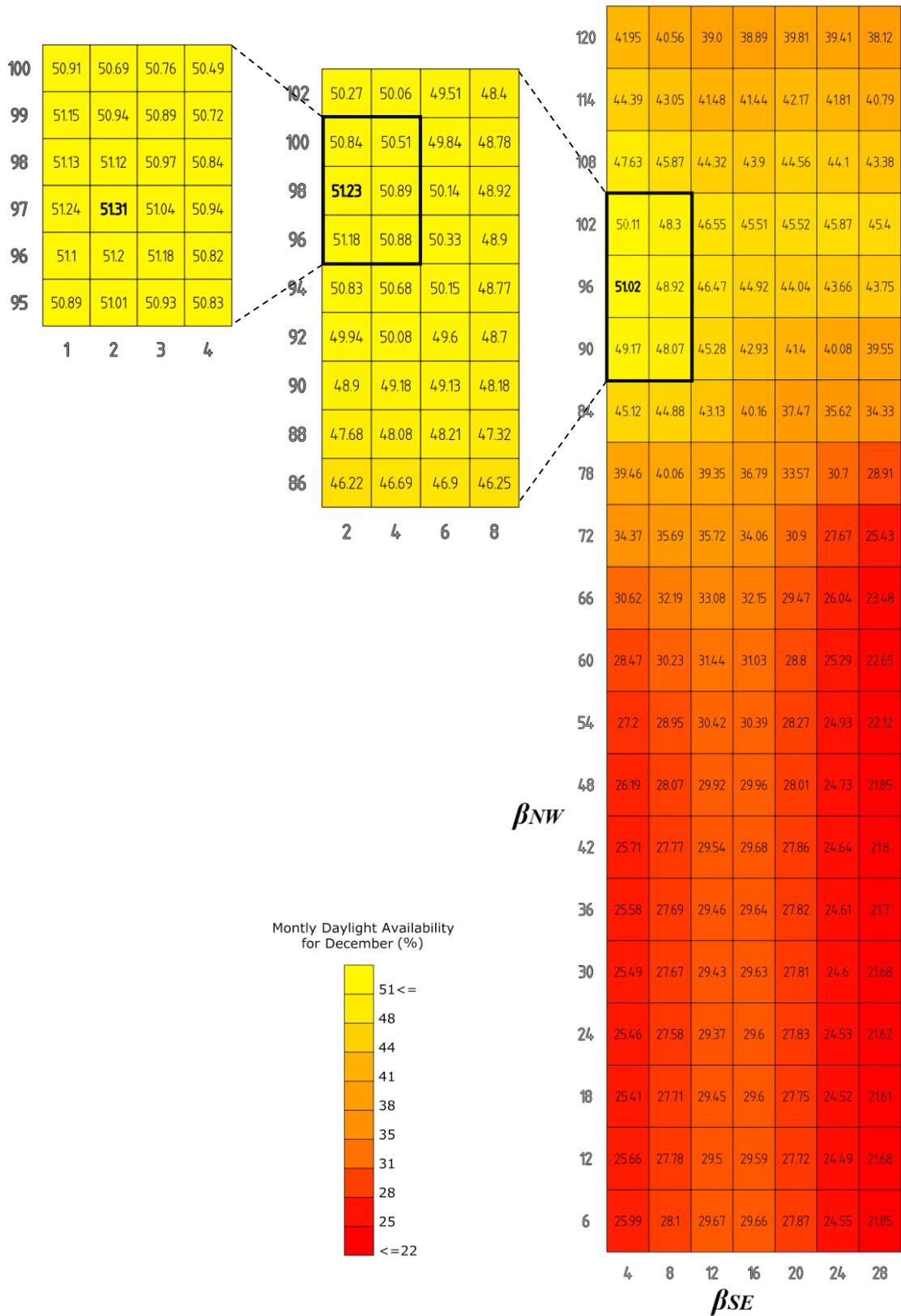
Figure 50. Finding Optimum Daylight Availability of the exhibition space during December through the parametric design exploration. Developed by the author in Grasshopper.
