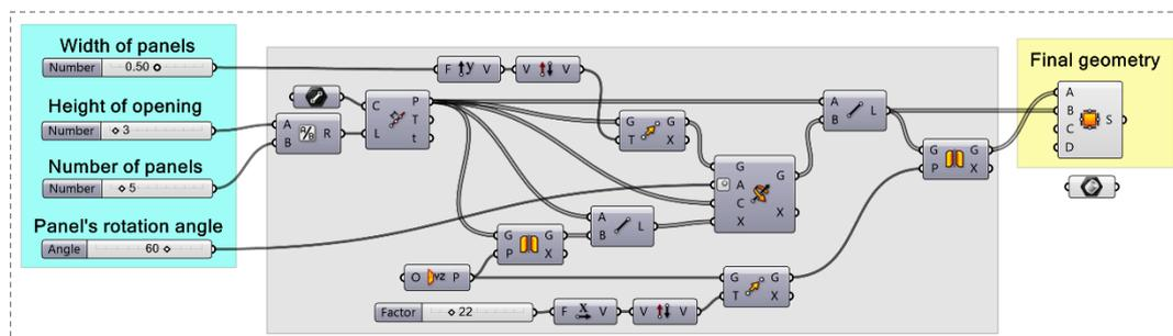
Figure 11. The design process of the horizontal louvered shading system in Grasshopper
