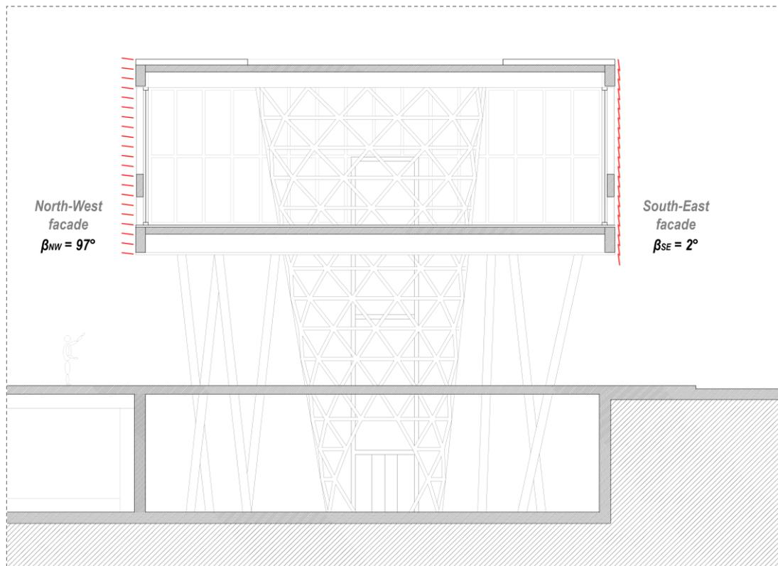
Figure 49. Optimum rotation angle of the panels to achieve the optimum daylight availability of the exhibition space during December.
