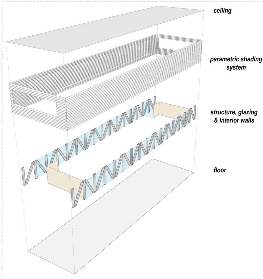
Figure 35. Different layers of building components that were modeled.
