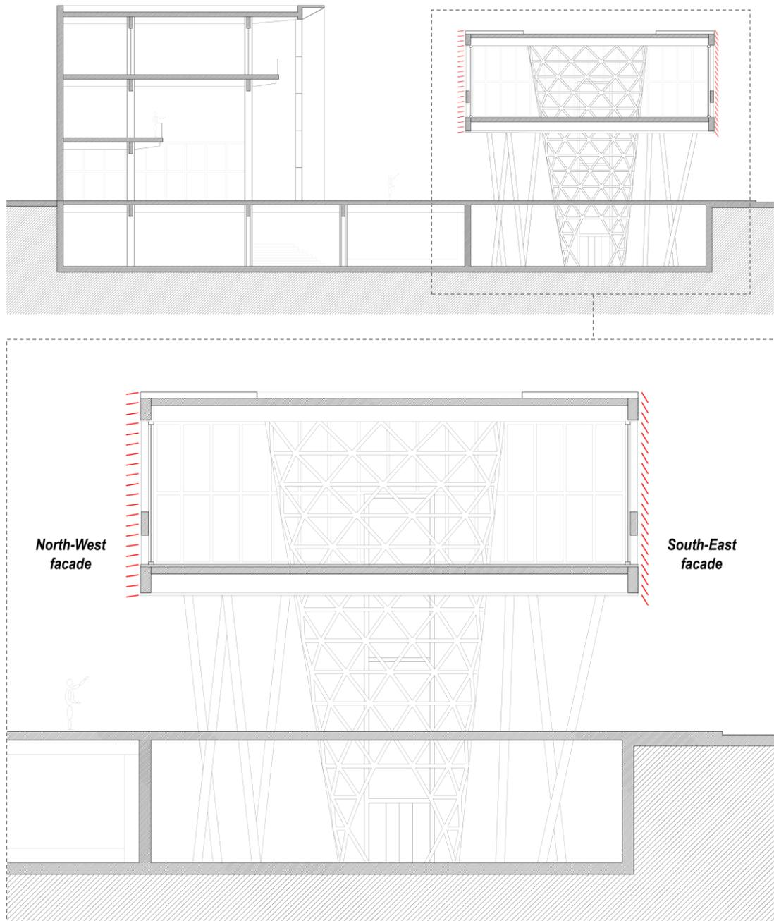
Figure 33. Cross section of the museum and the exhibition space, illustrating the individual performance of horizontal louvered shading panels on South-East and North-West façades.
