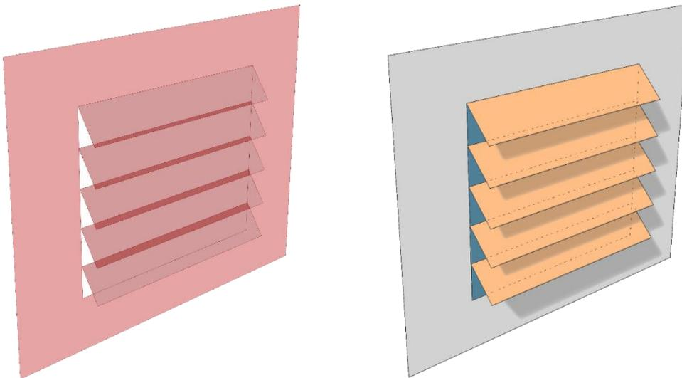
Figure 10. Horizontal louvered shading system that is designed parametrically in grasshopper.
