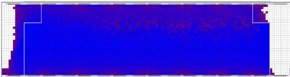
Figure 43. Desired daylight availability analysis within the exhibition space between the ranges of 0 to 250 lux. Prepared in Honeybee.
