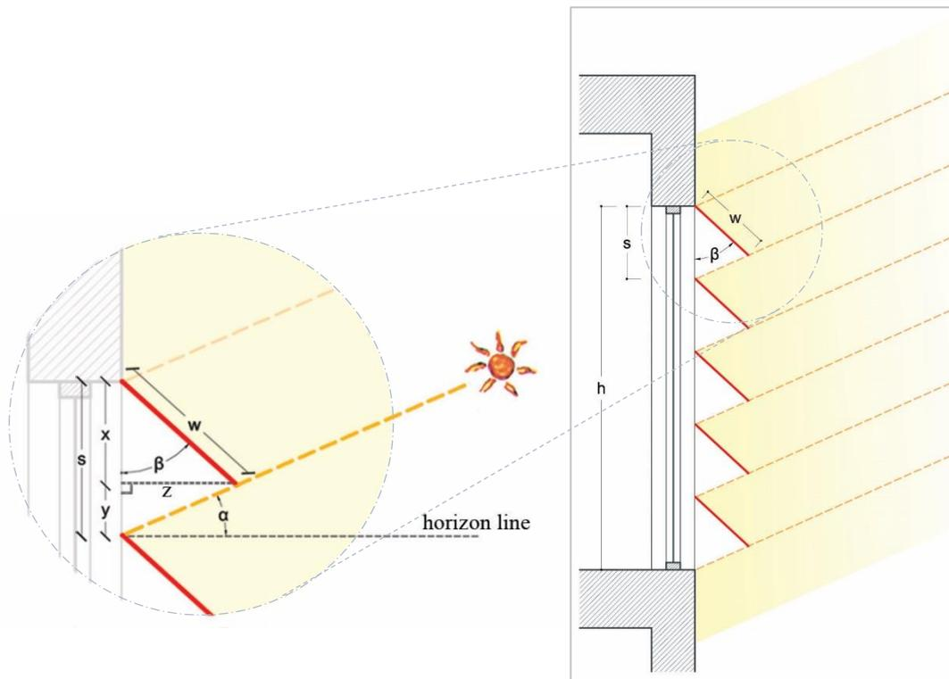
Figure 34. Design parameters of the horizontal louvered shading system.
