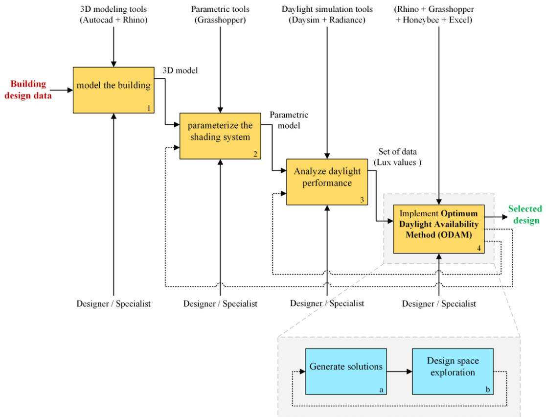
Figure 9. IDEF0 diagram of the design process
