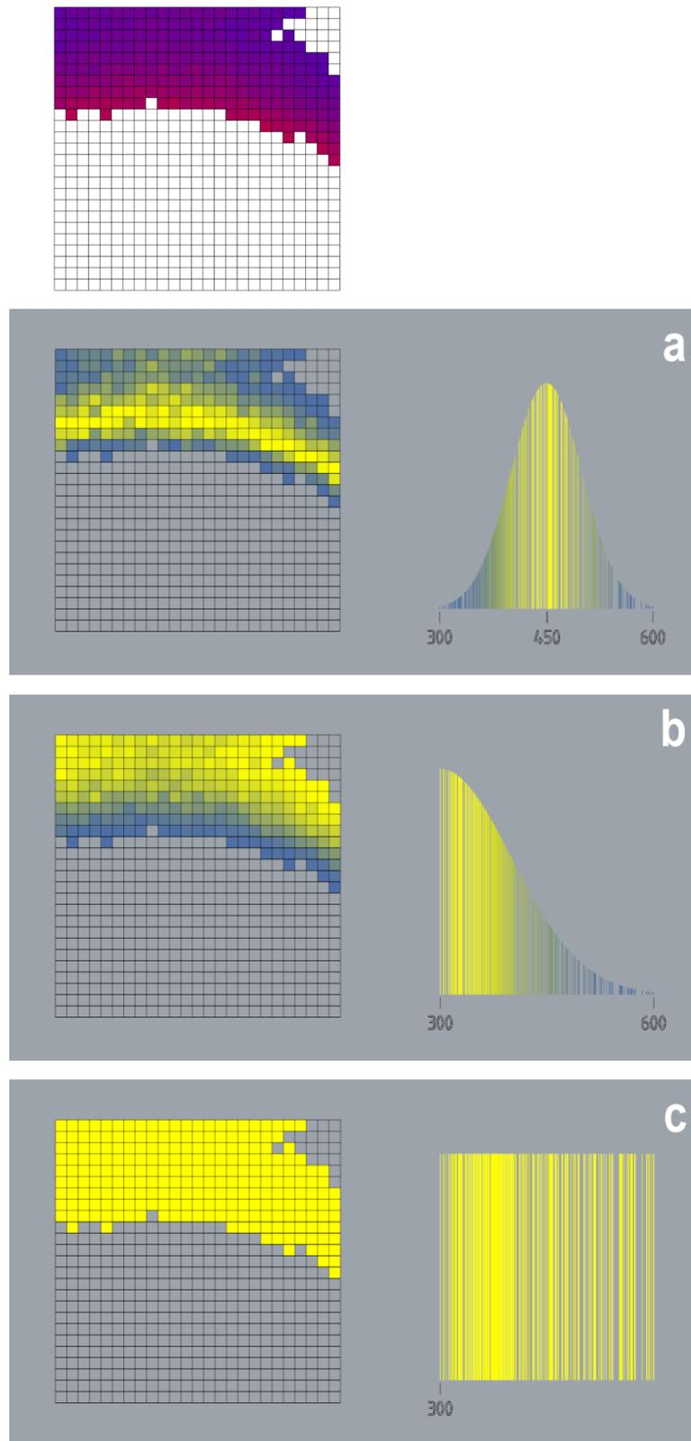
Figure 20. Fuzzy Gaussian membership values, assigned to the range of 300 to 600 lux in 3 different ways with respect to the desired visual task. Developed by the author in Grasshopper and Honeybee.
