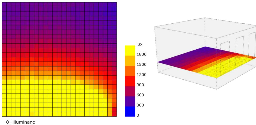
Figure 18. Sample room for evaluating daylighting performance, illustrating the level of illumination received by all grid cells on the working plane.
