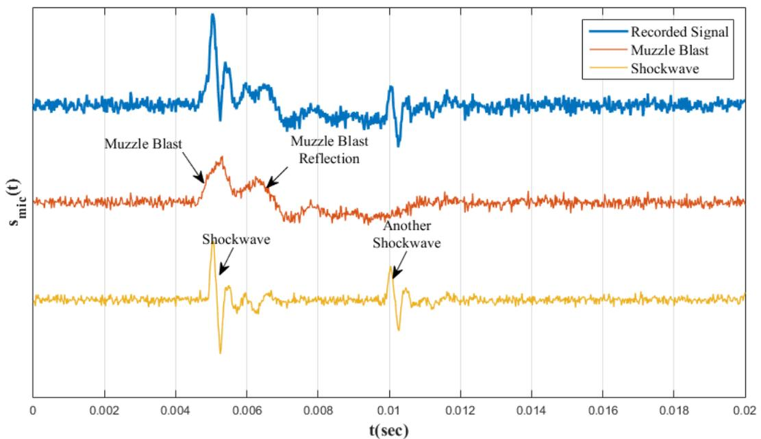
Figure 7.17: Example Recording of Multi Shot in a Single Frame
