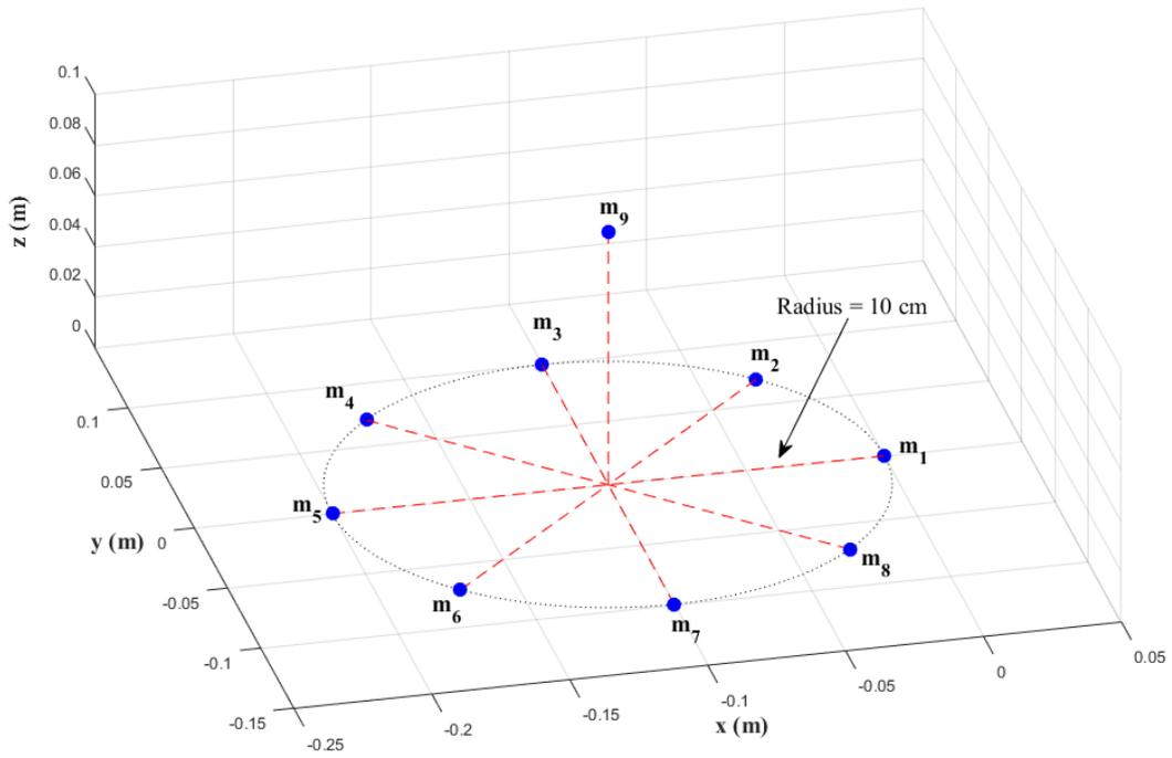
Figure 4.8: Microphone Array for WB-SRPBF Based DoA Estimation
