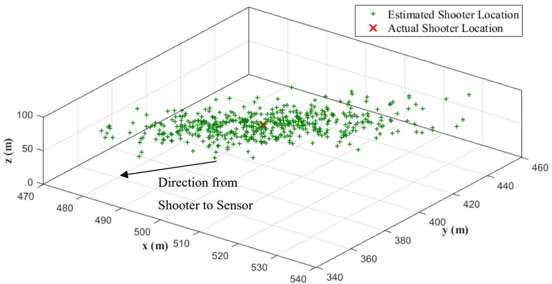
Figure 5.3: Effect of Microphone Position Error in Shooter Localization
