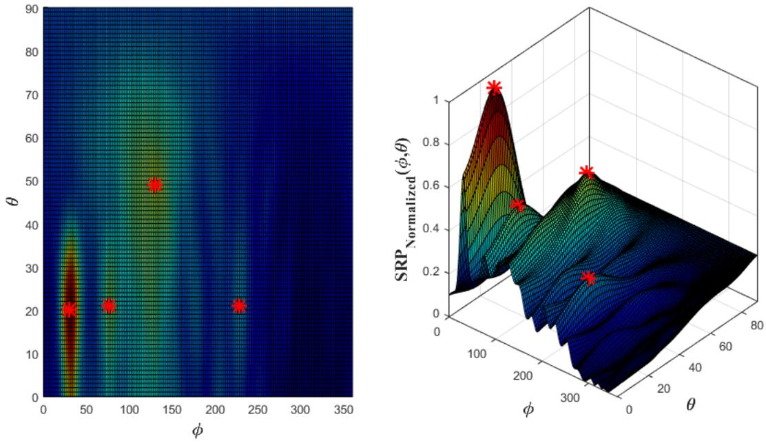
Figure 7.18: SRP Map for Multiple Shots with Reverberation (16 Microphone)
