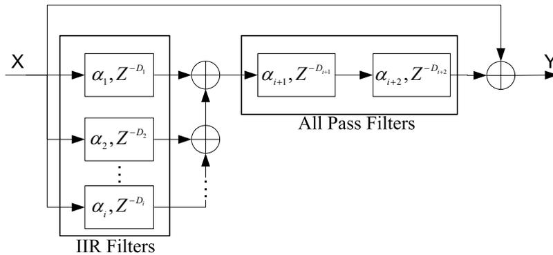
Figure C.2: Overall Block Diagram for Reverberation
