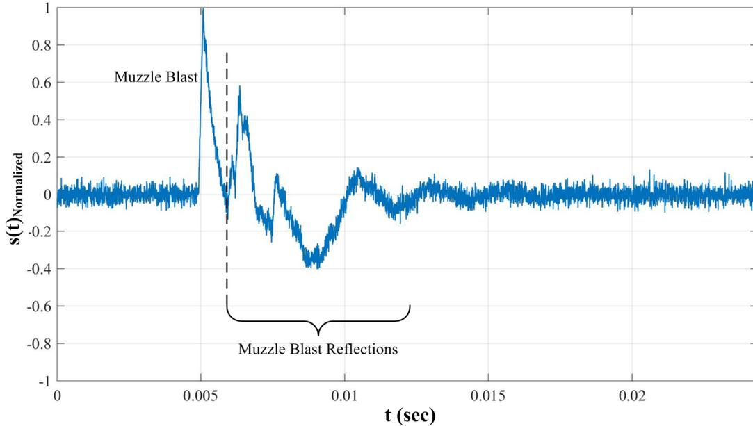
Figure 2.3: Muzzle Blast Signal with SNR of 10dB and Reflections
