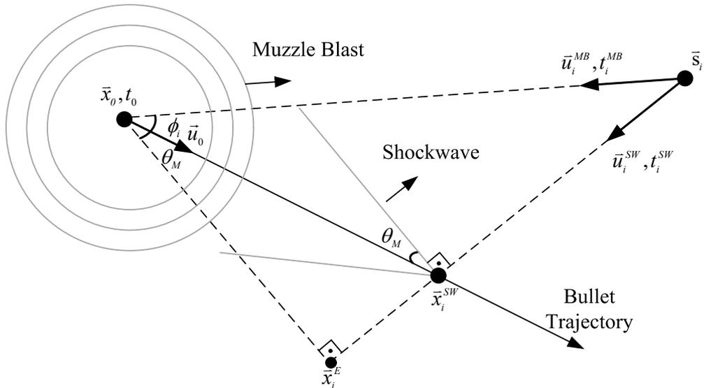
Figure 3.1: Geometry of Estimation Framework with respect to  $i^{\text{th}}$  Sensor
