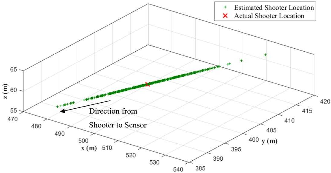
Figure 5.4: Effect of Speed of Sound Error in Shooter Localization
