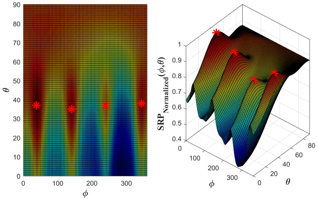
Figure 7.14: SRP Map of Uniformly Distributed Muzzle Blast (16 Microphone)
