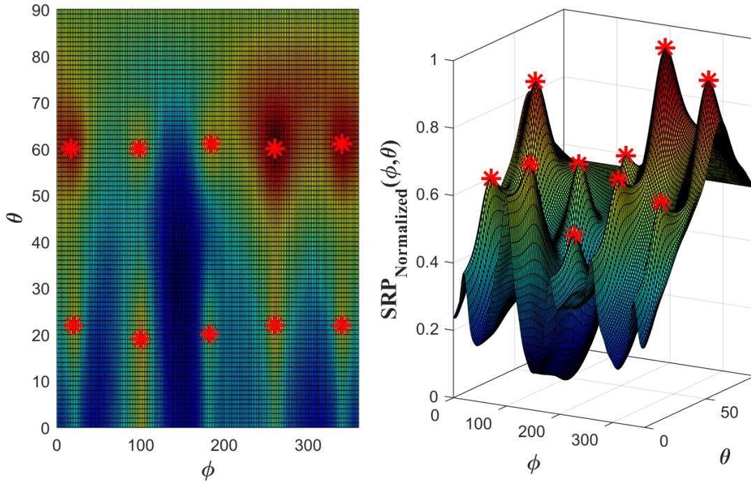
Figure 7.16: SRP Map of Uniformly Distributed Muzzle Blast (32 Microphone)
