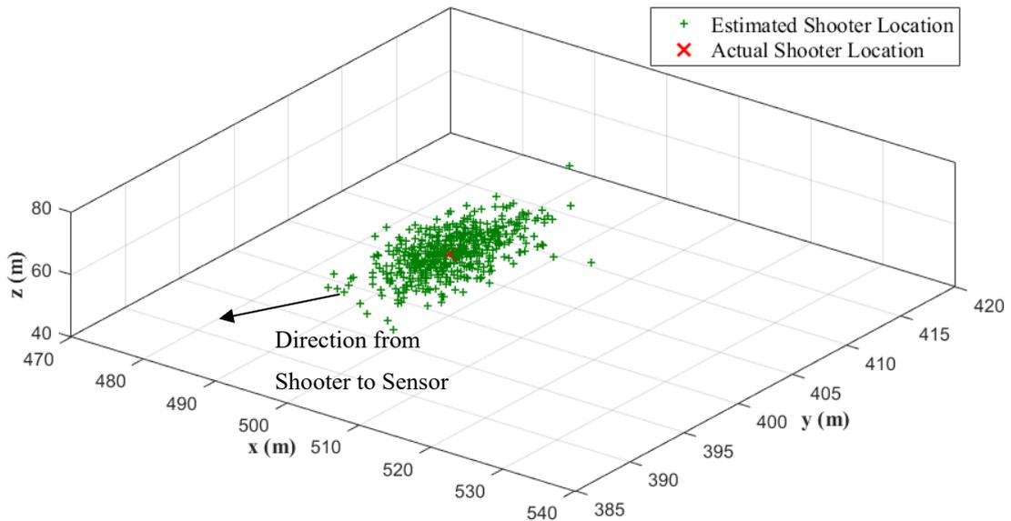
Figure 5.2: Effect of Sensor Location Error in Shooter Localization
