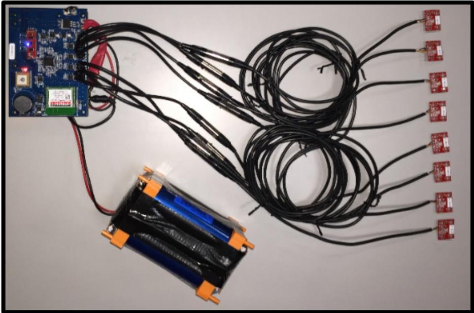
Figure 6.2: Hardware Design for Shooter Localization System
