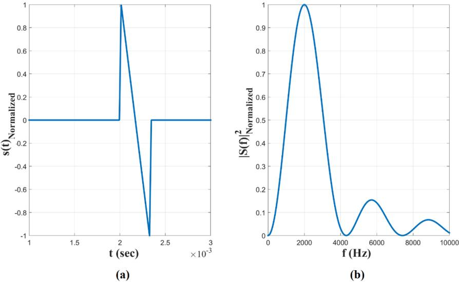
Figure 2.5: An Ideal Shockwave Signal in Time (a) and Frequency (b) Domains
