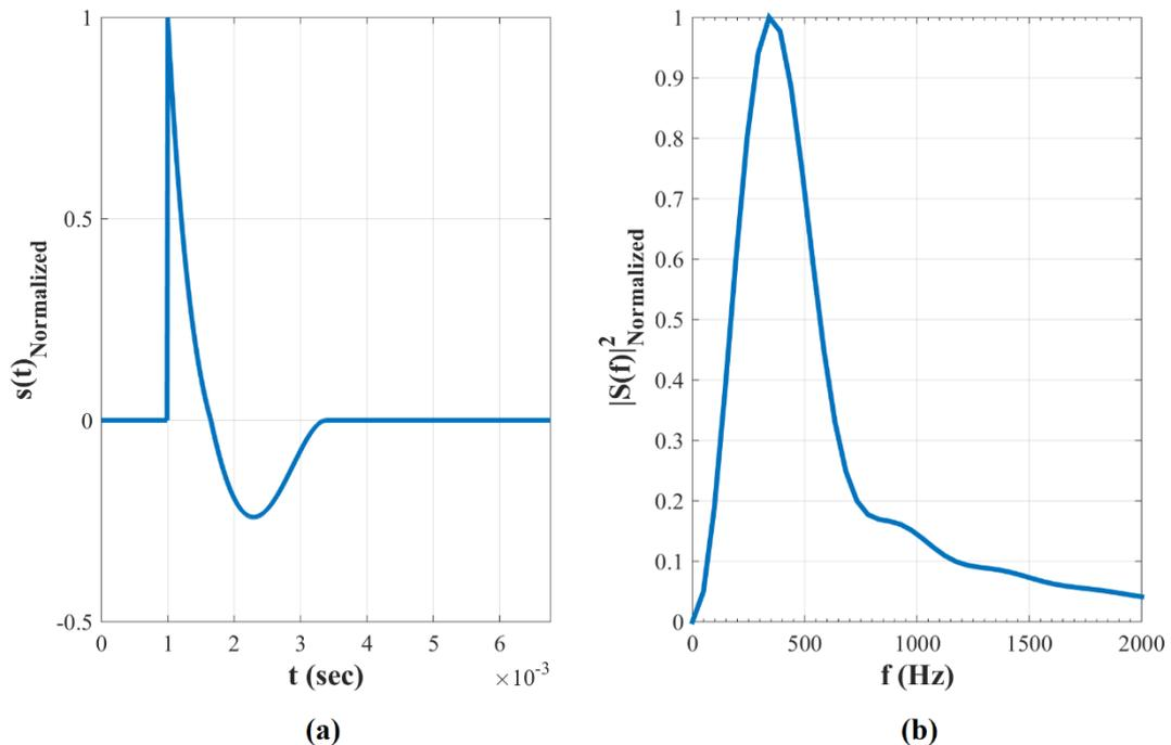
Figure 2.2: An Ideal Muzzle Blast Signal in Time (a) and Frequency (b) Domains
