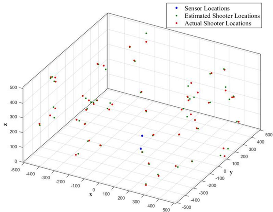
Figure 7.6: Shooter Localization with 3 Sensors – MB-SW Detection
