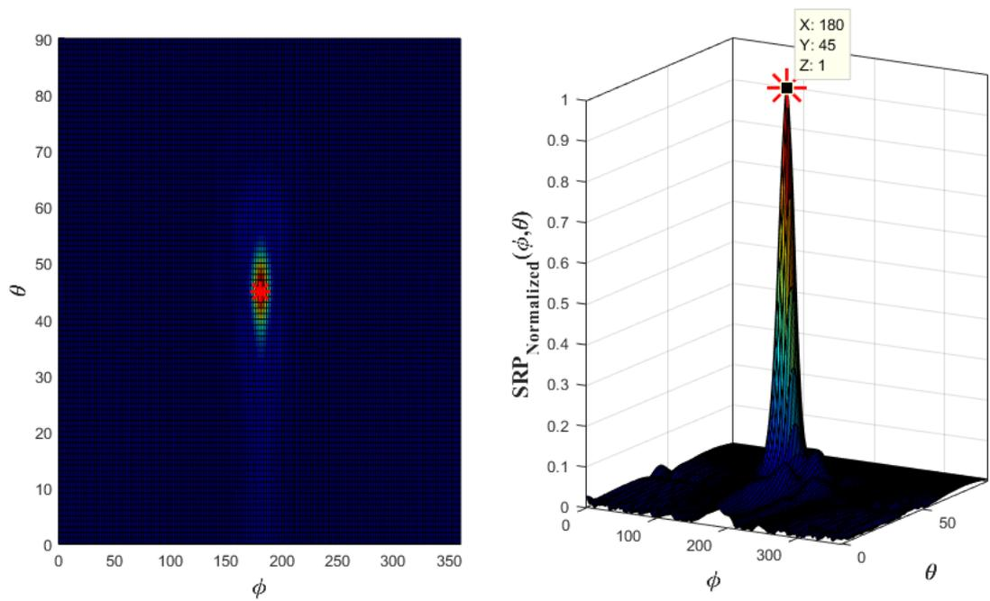
Figure 7.11: Beamwidth of Beamformer the Array of 32 Microphones
