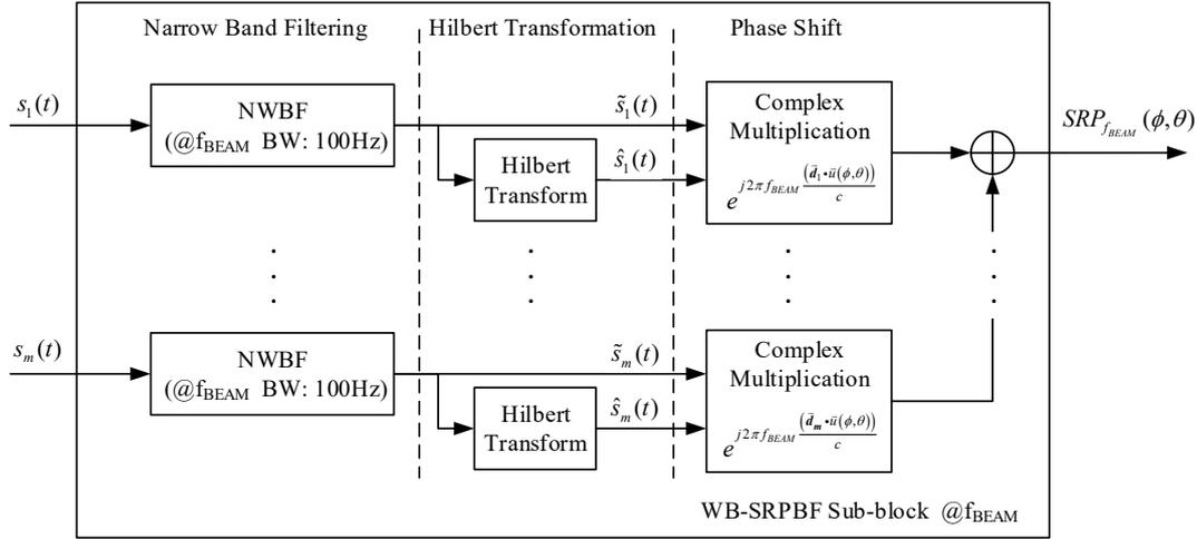
Figure 4.6: Block Diagram of Single Sub-Block of WB-SRPBF @  $f_{BEAM}$
