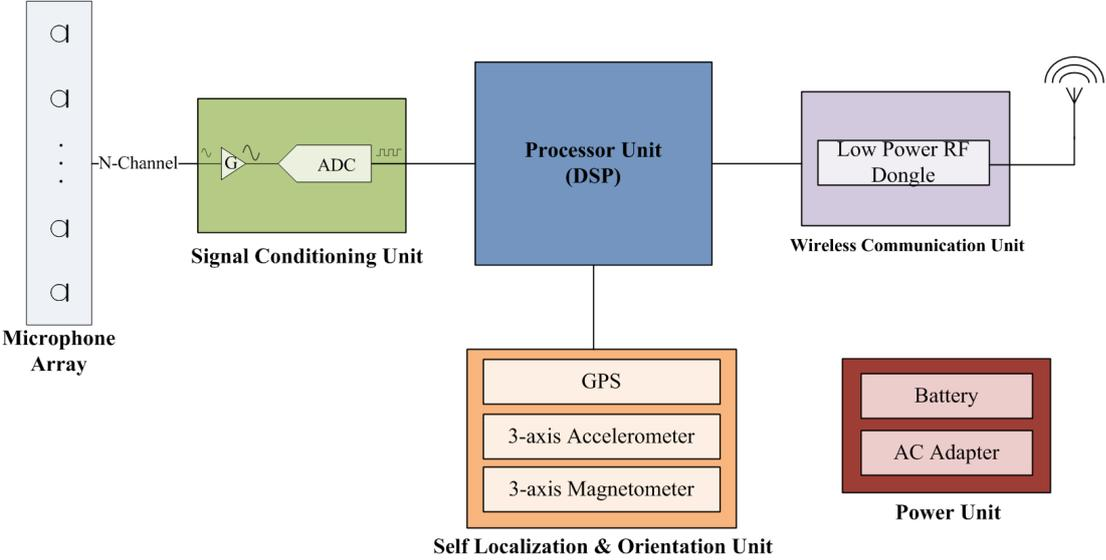
Figure 6.1: Hardware Architecture for Shooter Localization
