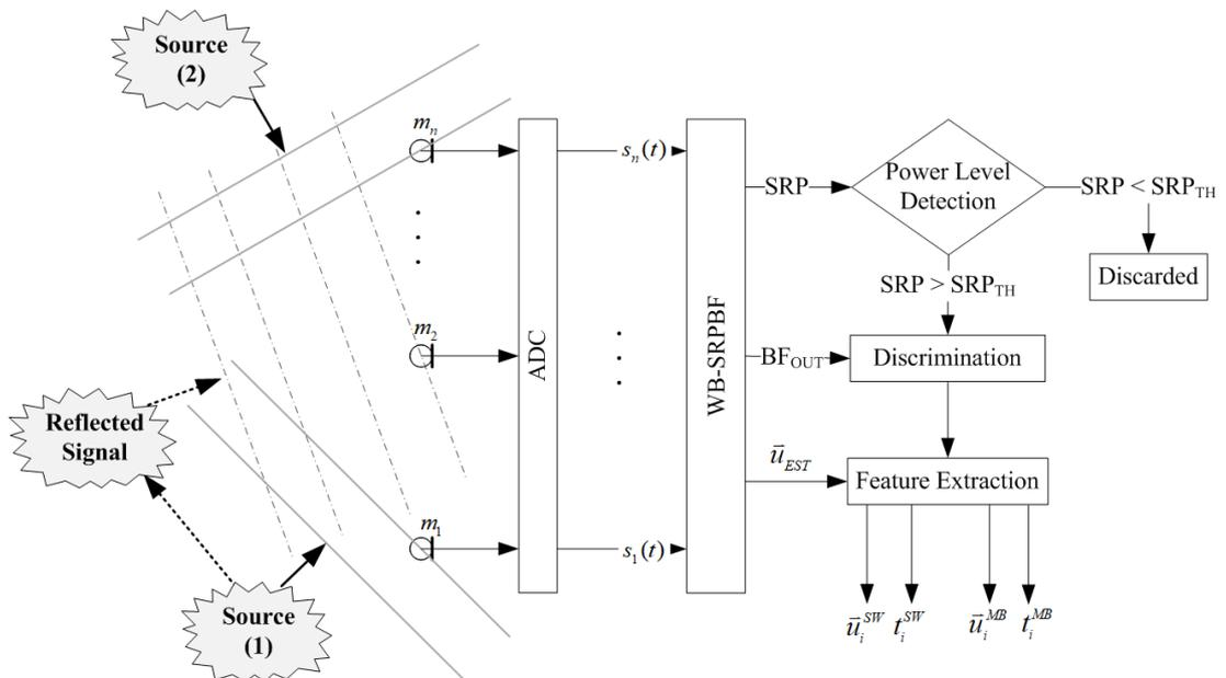
Figure 4.5: WB-SRPBF Block Diagram for Gunshot Acoustics
