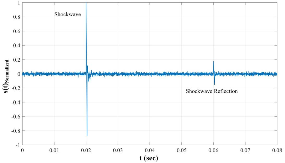
Figure 2.6: Shockwave Signal with SNR 10dB, and reflection
