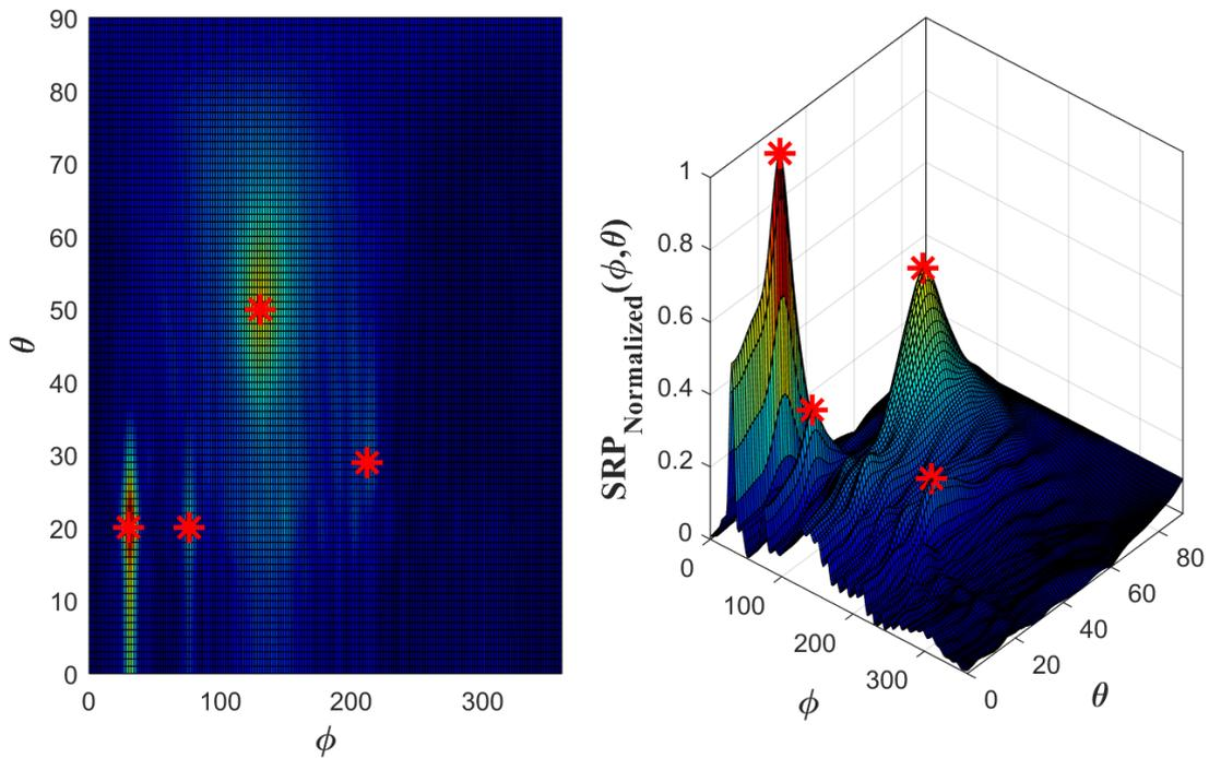
Figure 7.19: SRP Map for Multiple Shots with Reverberation (32 Microphone)
