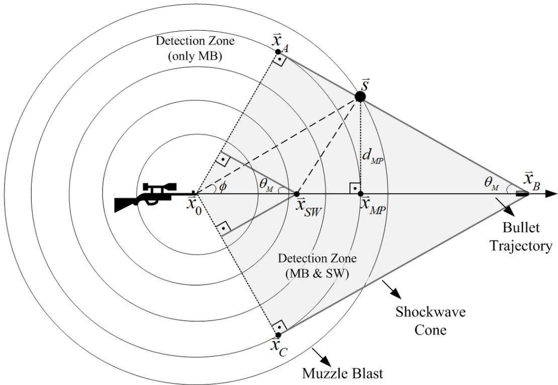
Figure 3.2: The Zones of Muzzle Blast and Shockwave in Gunshot Field
