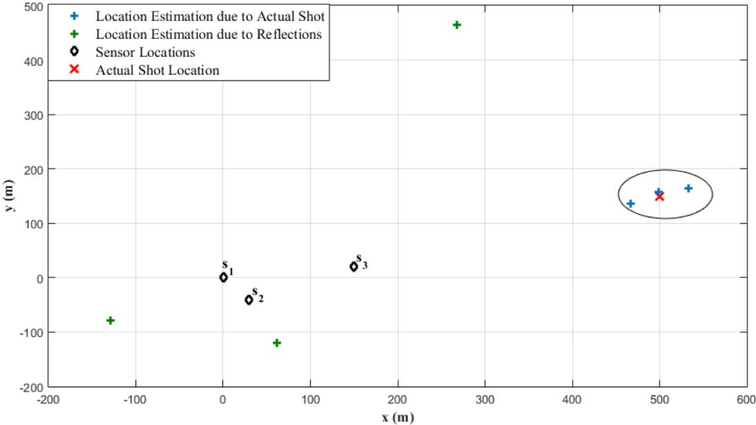
Figure 7.20: Example Reflection Elimination in Shooter Location Estimation
