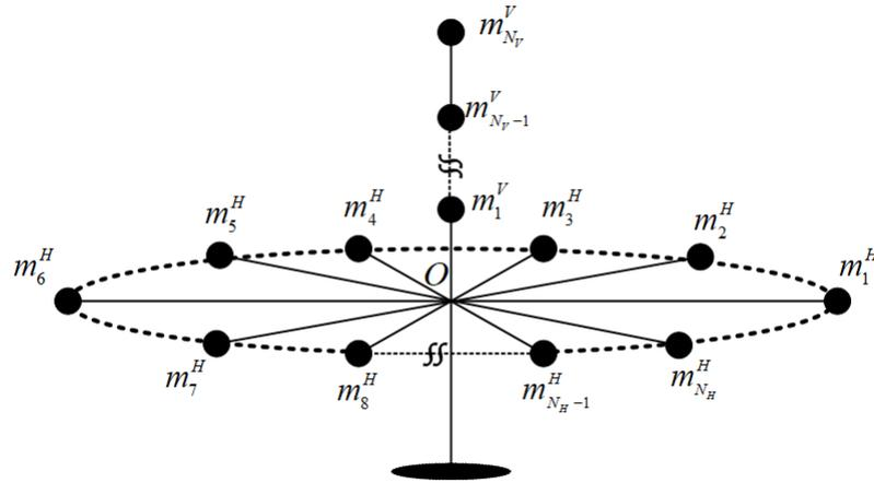
Figure 7.7: Microphone Array Topology for WB-SRPBF Technique
