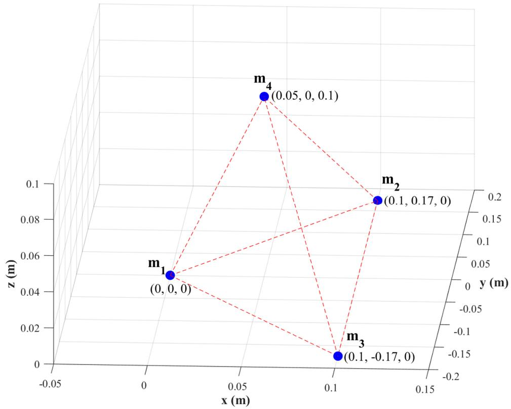
Figure 4.3: Tetrahedral Microphone Array for TDoA Based DoA Estimation
