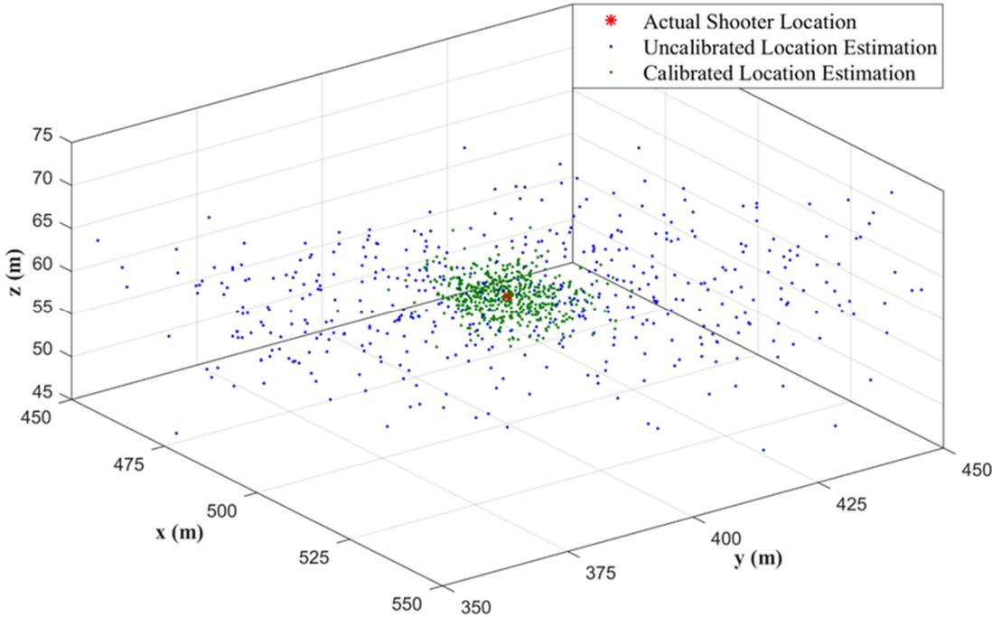
Figure 7.21: Calibrated and Uncalibrated Shooter Localization
