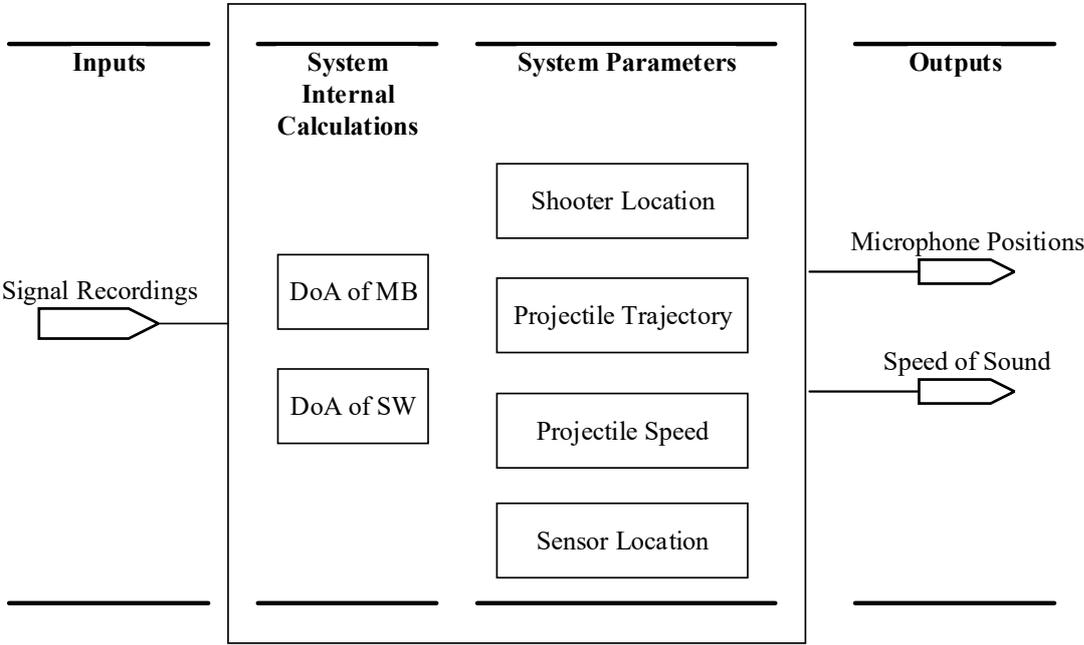
Figure 5.6: Acoustic Shooter Localization System Calibration Model
