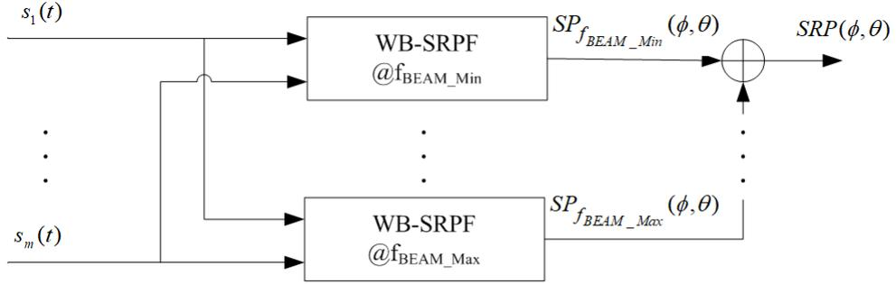
Figure 4.7: Block Diagram of Overall SRP Calculation in WB-SRPBF
