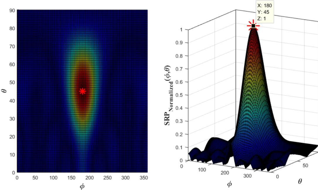
Figure 7.9: Beamwidth of Beamformer for the Array of 8 Microphones
