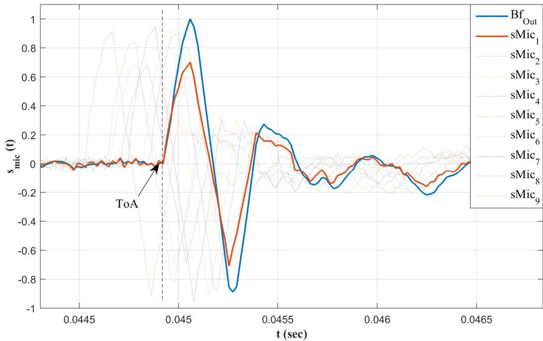
Figure 4.11: WB-SRP Beamformer Output for Erroneous DoA Estimation
