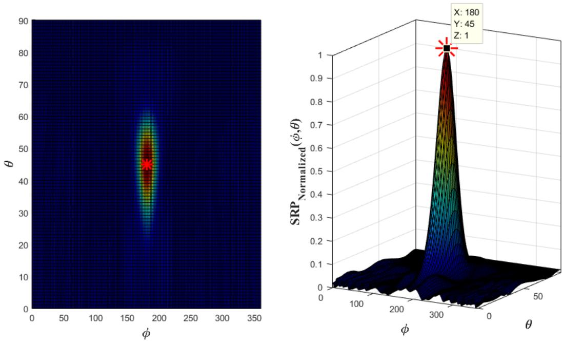
Figure 7.10: Beamwidth of Beamformer for the Array of 16 Microphones
