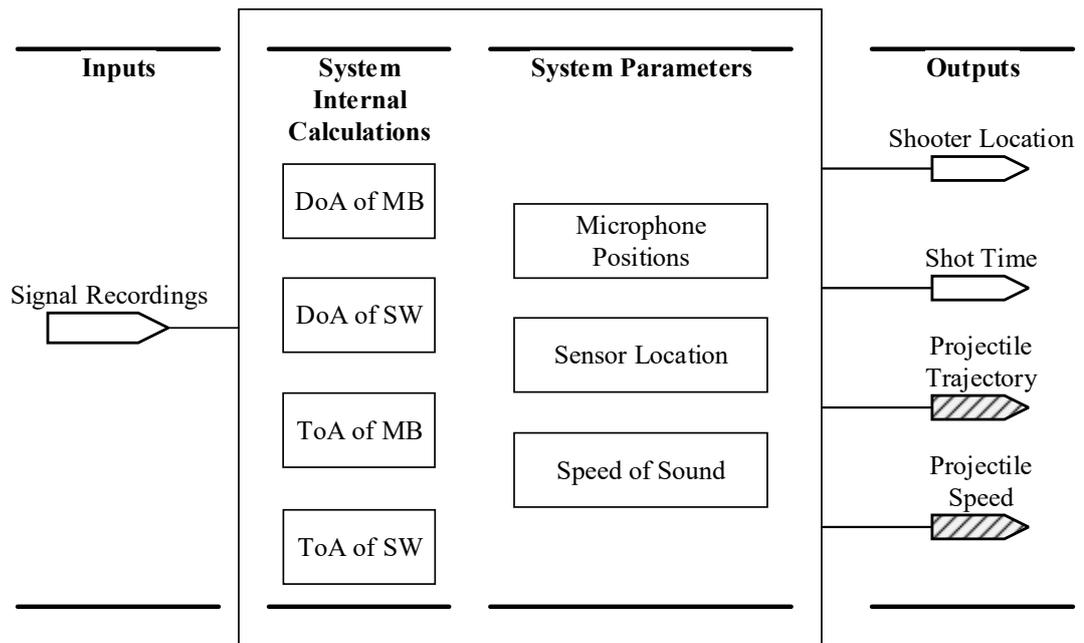
Figure 5.1: Acoustic Shooter Localization System Model
