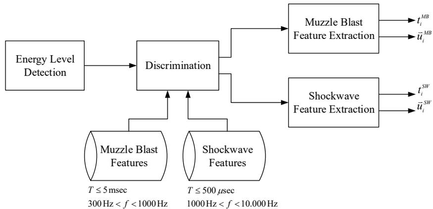
Figure 4.1: Block Diagram of Acoustic Event Analysis in a Sensor Node
