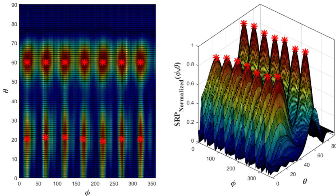
Figure 7.13: SRP Map of Uniformly Distributed Shockwave (16 Microphone)
