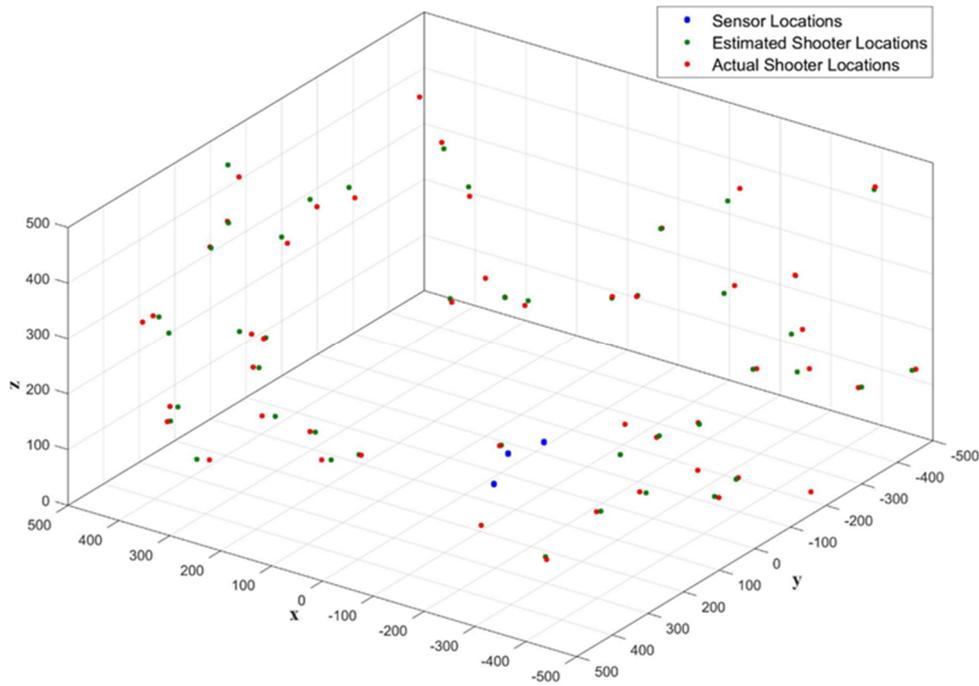
Figure 7.2: Shooter Localization with 3 Sensors – only MB Detection
