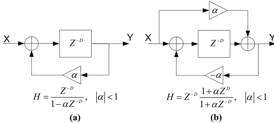
Figure C.1: Multiple Reflection IIR Filter (a) and All Pass Reverberator (b)
