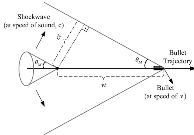
Figure 2.4: Shockwave Cone Geometry and Cone Angle
