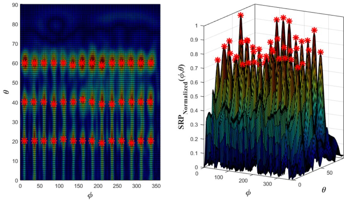
Figure 7.15: SRP Map of Uniformly Distributed Shockwave (32 Microphone)
