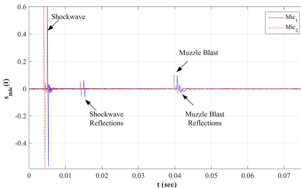
Figure 2.1: Gunshot Acoustic Events – Muzzle Blast and Shockwave
