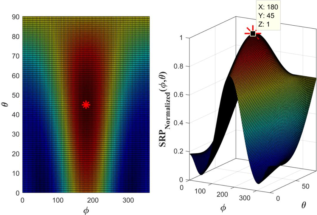
Figure 7.8: Beamwidth of Beamformer the Array of 4 Microphones
