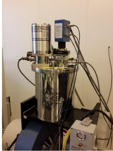
Figure 3.3 He cryostat used for dark current measurement.
