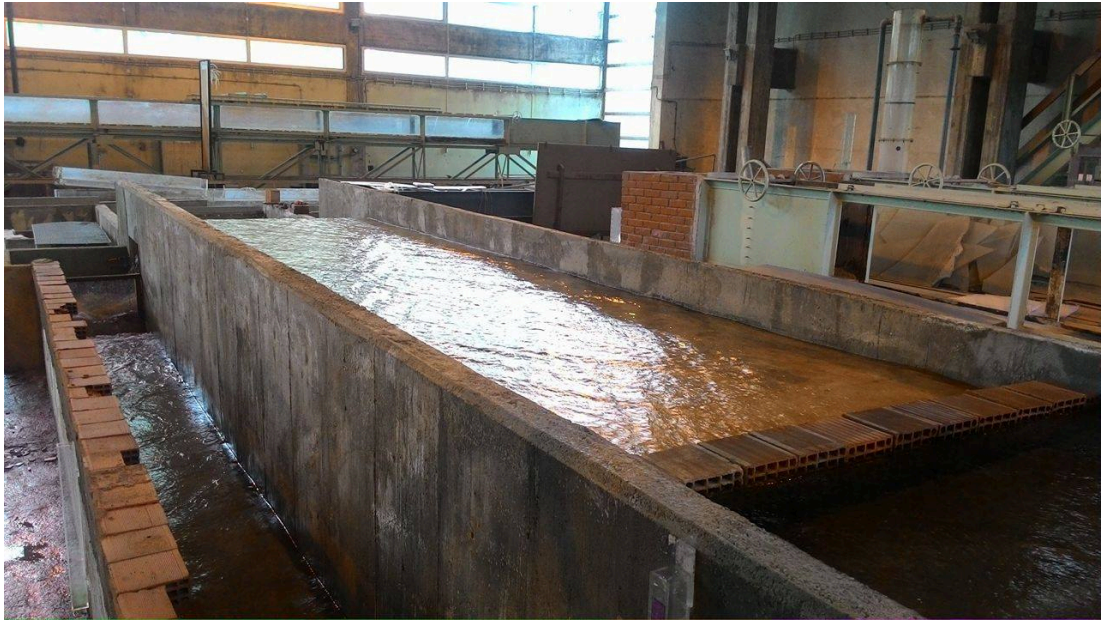
Figure 3.2 View of the Tyrolean weir model from upstream
