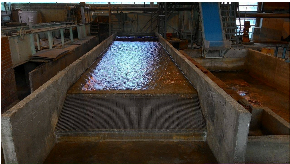
Figure 3.3 View of the main channel and Tyrolean screen from downstream
