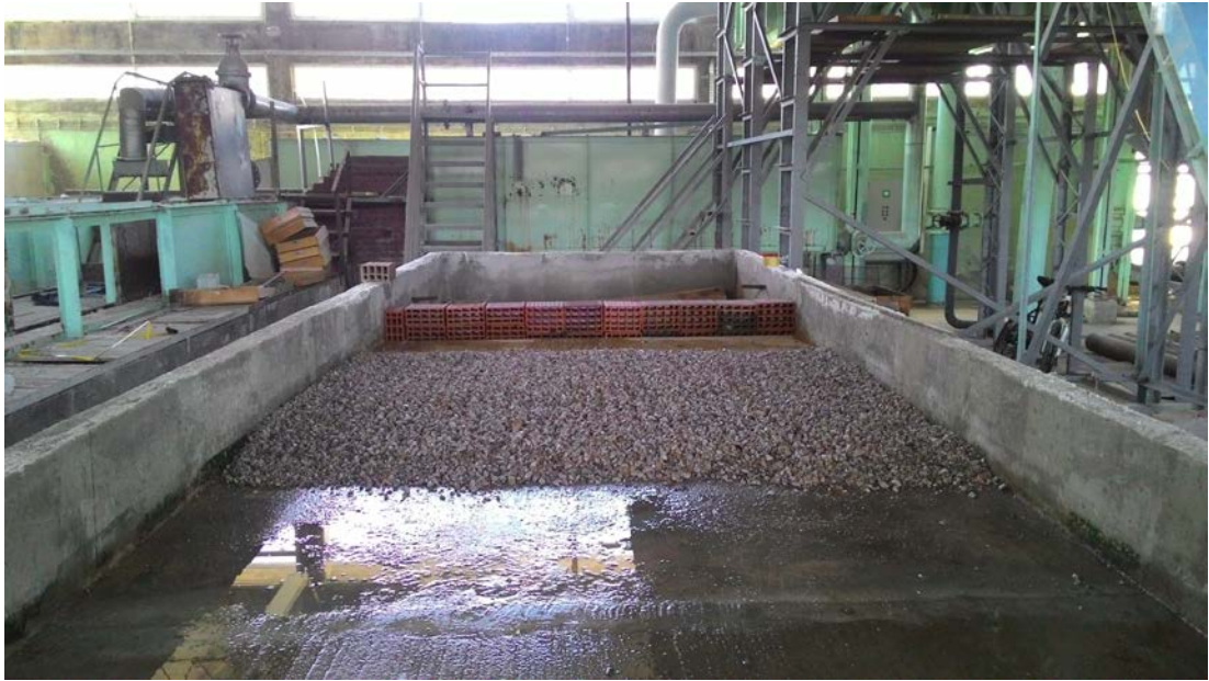
Figure 3.8 View of the sediment mixture used in the experiments to investigate sediment capture rate of the trash rack
