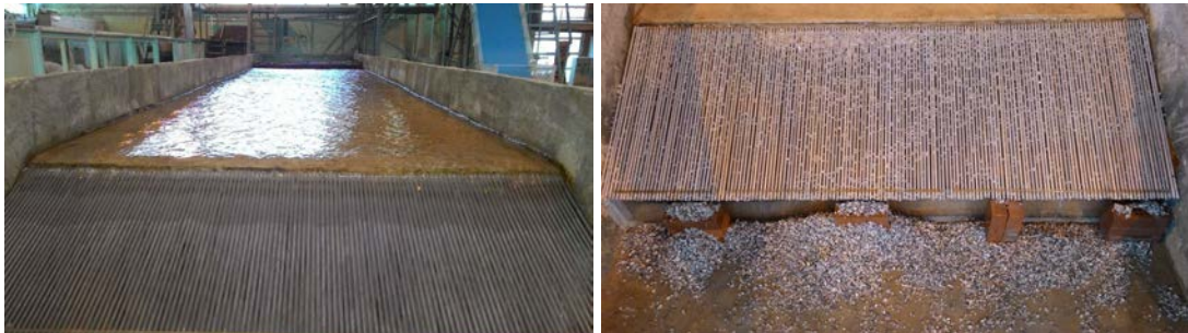
Figure 3.9 Clean and clogged Tyrolean screen with clearance of e=3 mm
