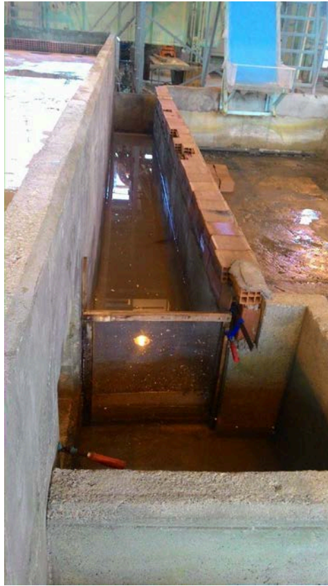
Figure 3.5 Sediment trap reservoir and side channel
