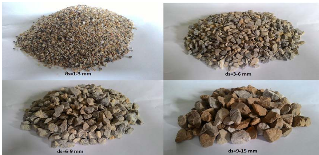
Figure 3.7 Different sizes of sediment used in the experiments
