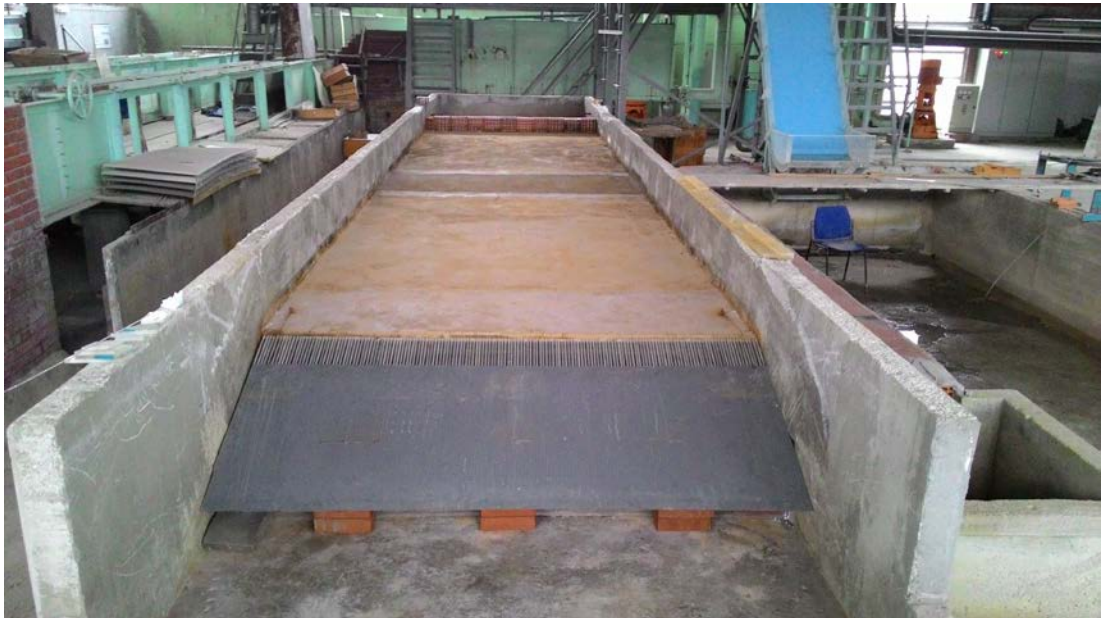
Figure 3.6 View of the steel plate used in the arrangement of the trash rack length
