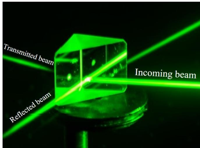
Figure 3.1: The direction of reflected and transmitted beams. Adapted from [54]
