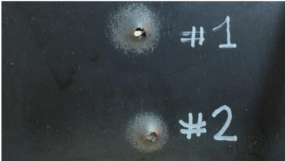
Figure 67 Rear Surface of The Impacted 2-2 Configuration (Back of Second Layer)
