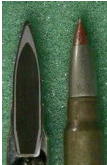
Figure 3 7.62 mm AP Bullet Cut View [21]
