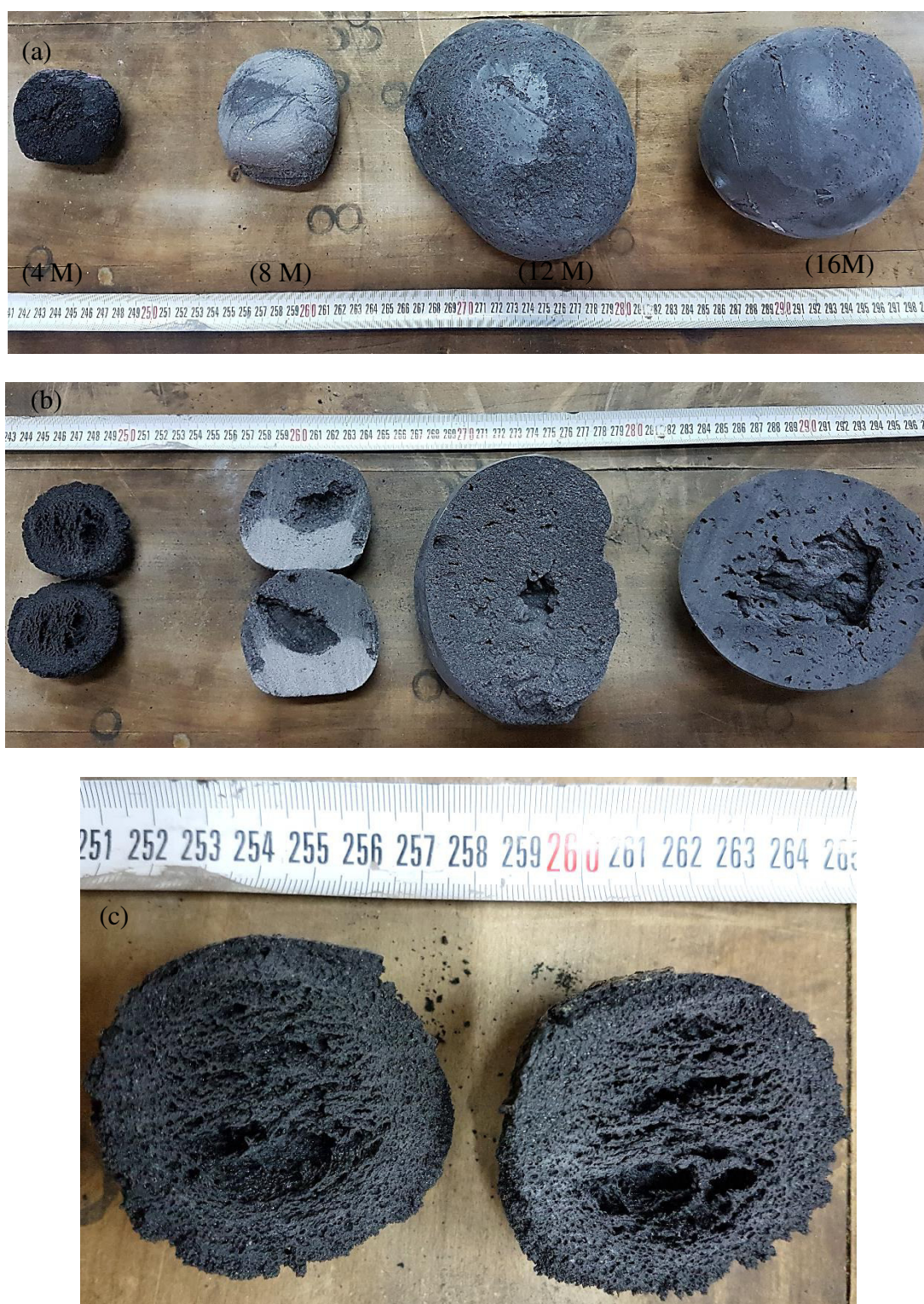
Figure 4.1 (a) Size comparison of different solution concentrations, (b) cross section of different solution concentration, and cross section of (c) 4 M, (d) 8 M, (e) 12 M, and (f) 16 M.
