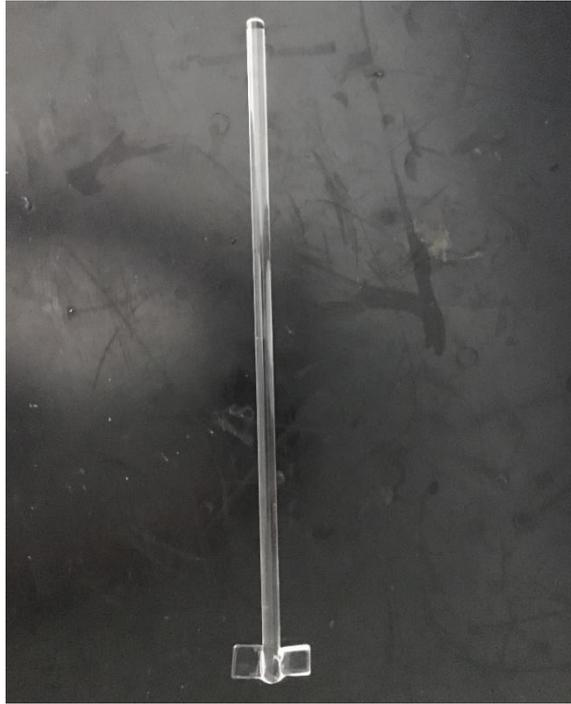
**Figure F-5: Matest propeller**
