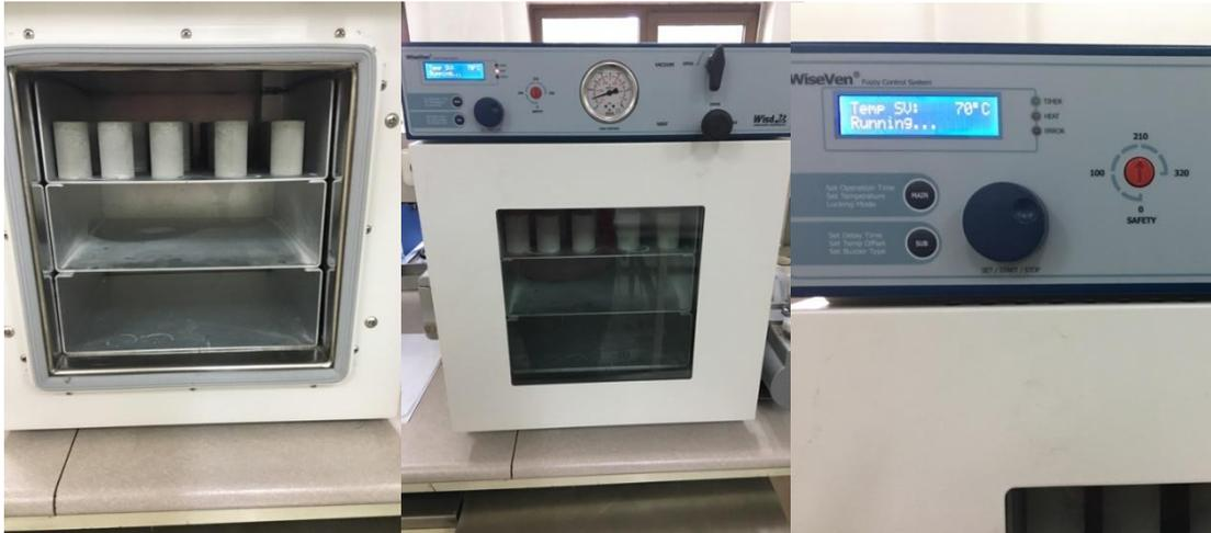
**Figure 5-5 : Removing moisture inside the core specimens by using vacuum oven**
