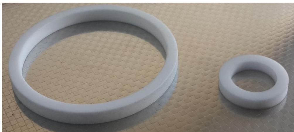
Figure 3. 1 PTFE rings used as a deformable die. Smaller diameter ring on the right was used for preliminary experiments. While the one on the left was used to fabricate 2 inch diameter \text{La}_{0.8}\text{Sr}_{0.2}\text{CoO}_{3-\delta} (LSC-113) sputter gun.
