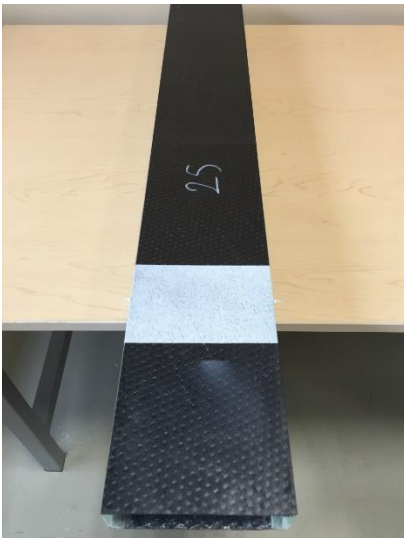
Figure 2.30 GFRP/CFRP hybrid box-beam structure having 25^\circ fiber orientation angle in the upper and lower CFRP flanges
