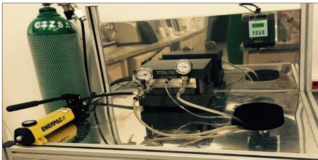
Figure 9. Membrane filtration system used for the experiment
