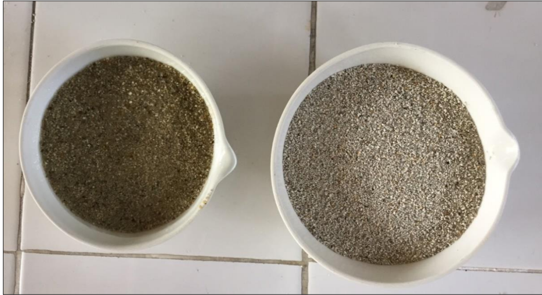
Figure 7. Zeolite samples before (left) and after (right) drying
