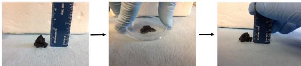
Figure 2.23: Resiliency of covalently linked graphene oxide-PEGMEMA under load 140 .
