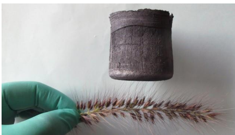
Figure 1.2: A graphene oxide based aerogel with low density 12 .
