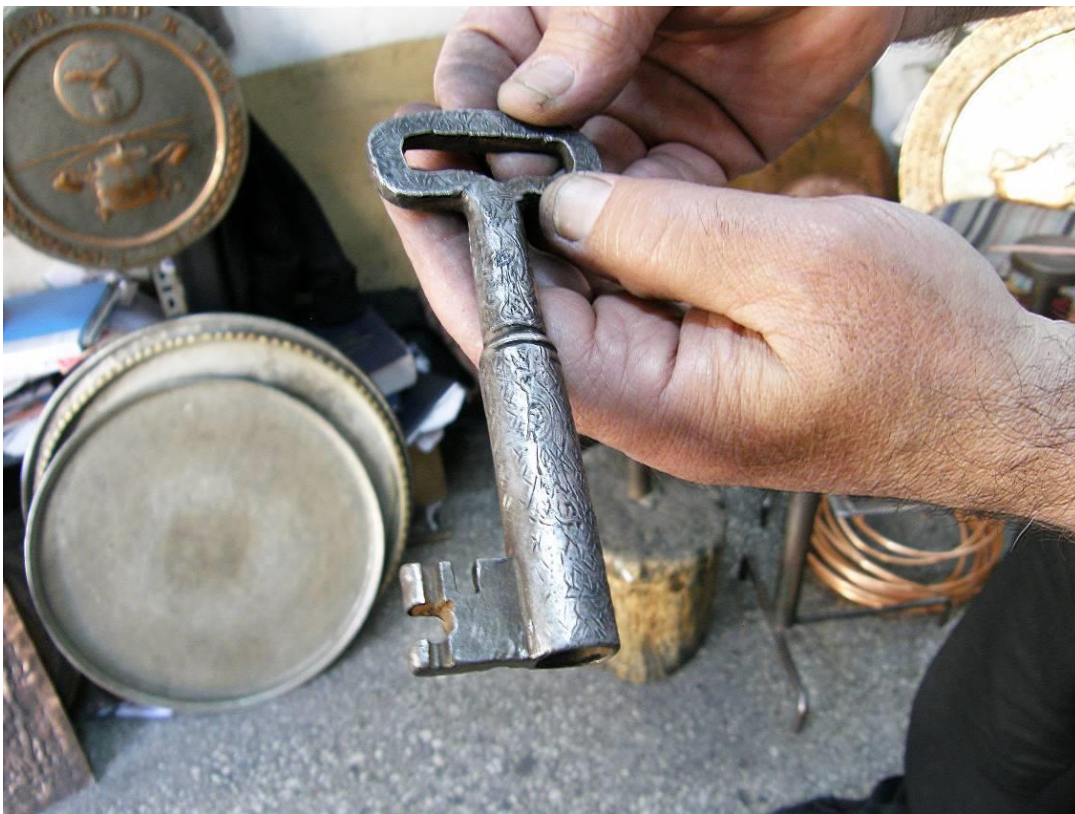
Figure 4.33: An old key on which the craftsman applied surface embellishment by using the engraving technique.
