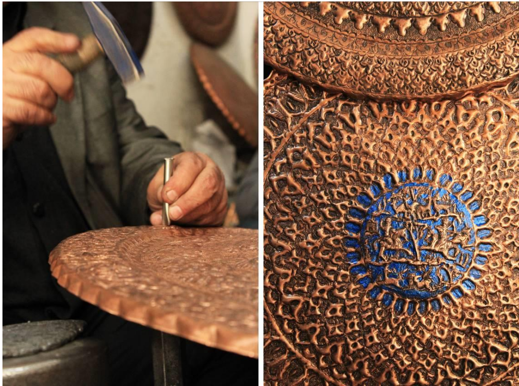
Figure 4.27: ( left ) The craftsman using a steel chisel and hammer; ( right ) close-up of an elaborate relief work.
