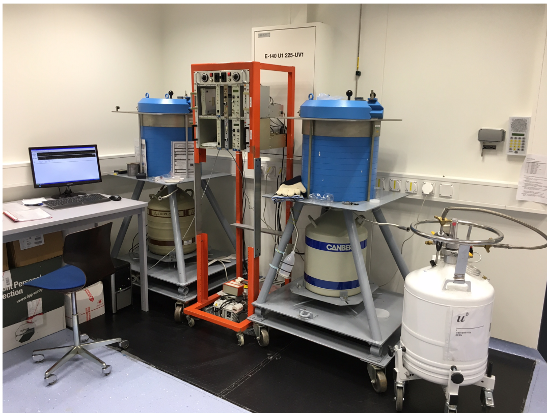
Figure 4.21: Two germanium detectors in the Bern medical cyclotron laboratory
