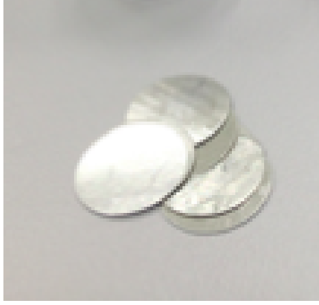
Figure 4.2: Aluminum foils as the energy degrader
