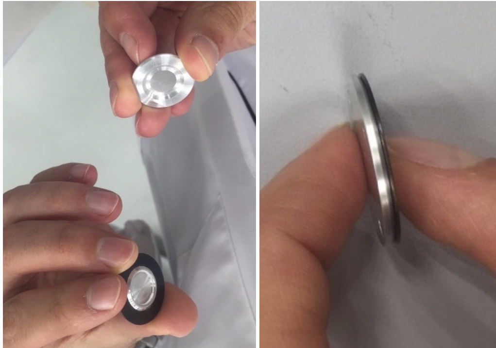
Figure 4.14: Open (left), and closed (right) representation of the target holder
