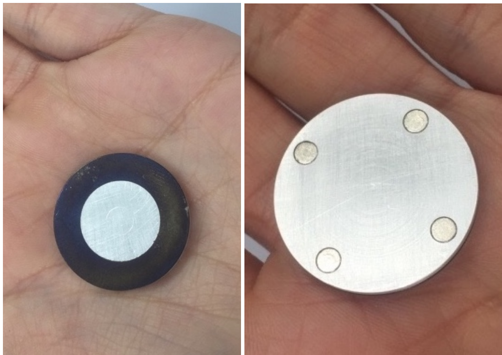
Figure 4.15: Front side (left), and back side of the target holder and the magnets on it (right)
