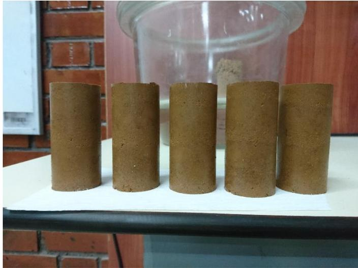
**Figure 3.32. Cylindrical specimens prepared for both split tensile testing and unconfined compression testing**
