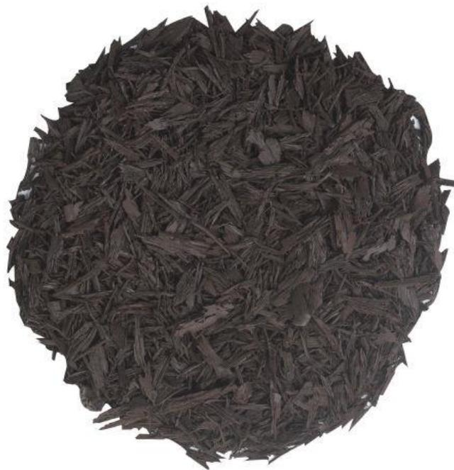
**Figure 2.31. An example of shredded rubber waste (Adopted from [www.acehardware.com](http://www.acehardware.com))**
