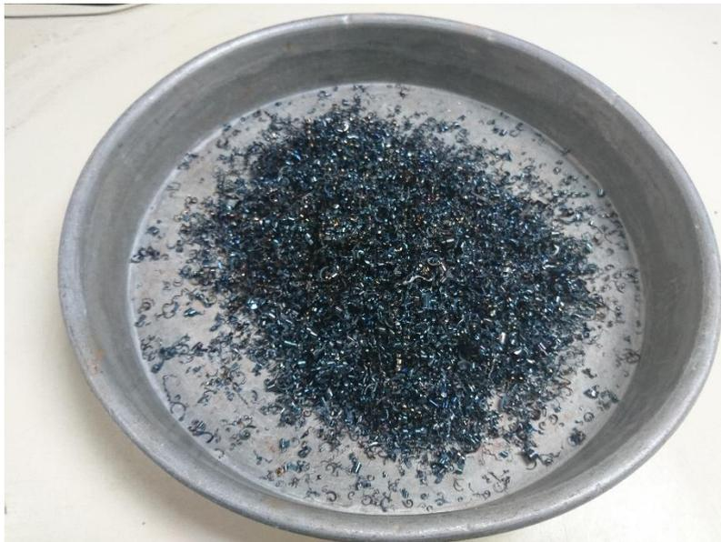
**Figure 3.9. Waste metal swarf which was used in this study**
