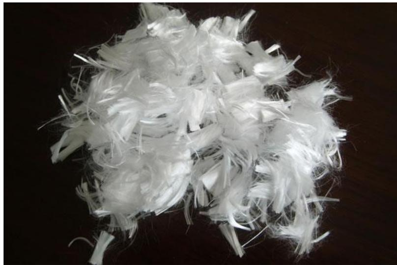
**Figure 2.27. An example of polyester fiber which is used for tensile strength stabilization and improvement (Adopted from [www.polyrope-fence.com](http://www.polyrope-fence.com))**
