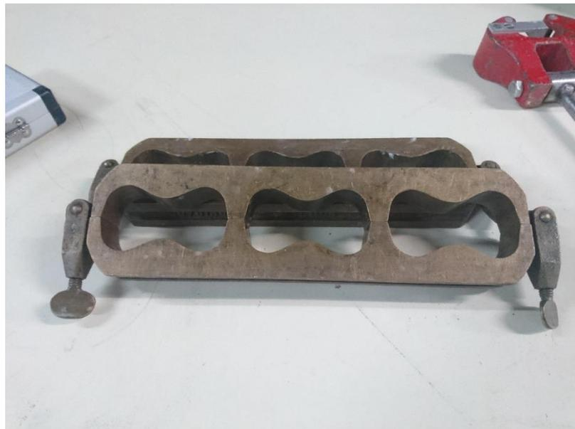
**Figure 3.23. Compaction mold which was used in this study to prepare 8-shaped specimens**
