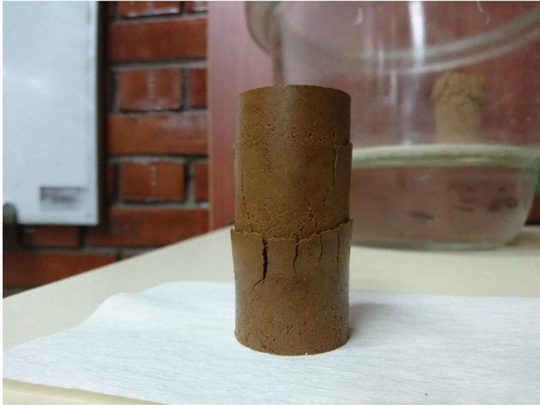
**Figure 4.16. Unconfined compression test specimen of AC-01 mixture after the testing process**
