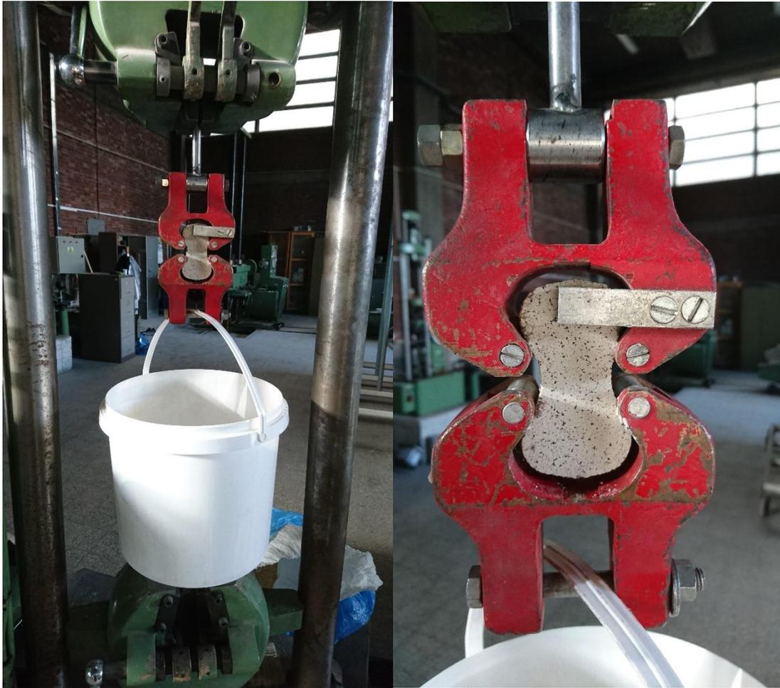
**Figure 3.29. Direct tensile testing set up which was developed and used in this study**
