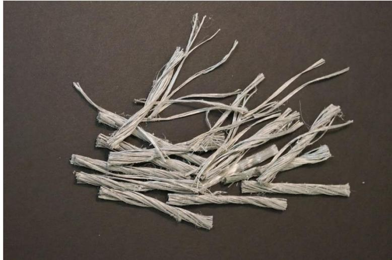
**Figure 2.26. An example of polypropylene fiber which is used for tensile strength stabilization and improvement (Adopted from [www.fortaferro.com](http://www.fortaferro.com))**
