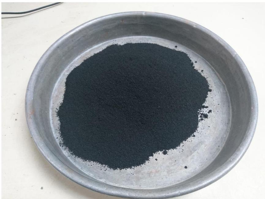
**Figure 3.11. Pulverized rubber which was used in the experiments**
