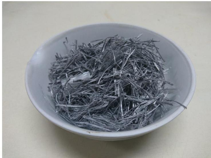
**Figure 3.8. Final form of the synthetic fiber which was used in this study**
