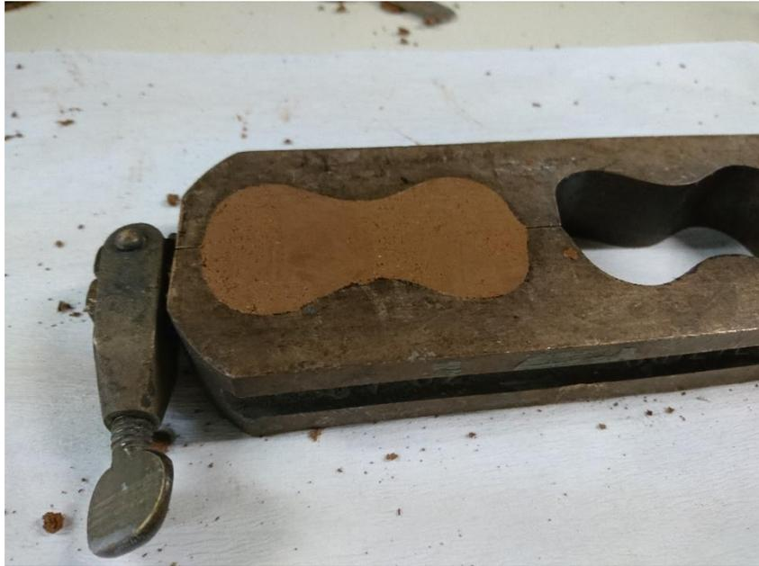
**Figure 3.26. Specimen after compaction process in the mold**
