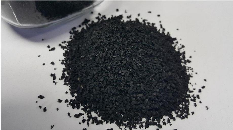
**Figure 2.32. An example of crumb rubber waste (Adopted from [www.continenetal-platform.com](http://www.continenetal-platform.com))**
