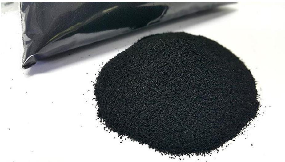
**Figure 2.33. An example of pulverized rubber waste (Adopted from [www.continenetal-platform.com](http://www.continenetal-platform.com))**
