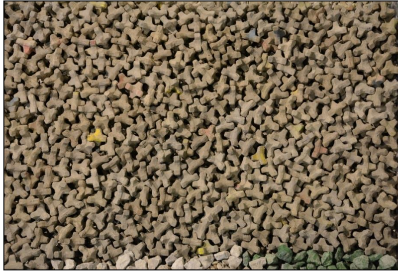
Figure 6.32 Accropode II Placement in Experiment Section
