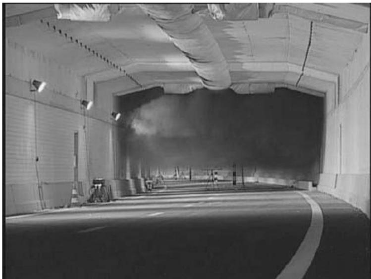
**Figure 2.3.** Propagating smoke in Benelux experiments [43]
