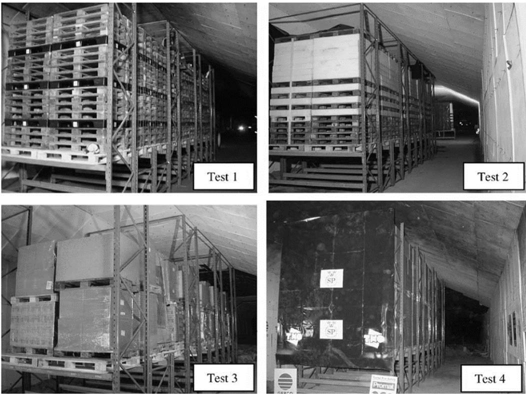
**Figure 2.5.** Test commodity used in large-scale tests of Runehamar tunnel [44]
