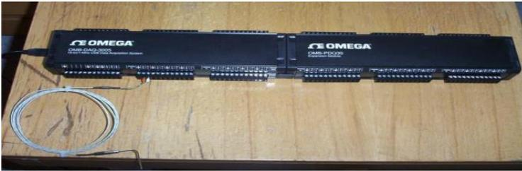
**Figure 3.4.** Data acquisition pack with connected thermocouple
