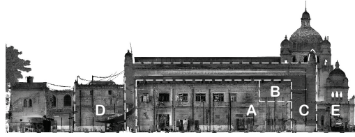
Figure 3.25: Lahore Museum— Eastern Façade (2016) Orthographic projection from laser scan point-clouds. A: Laboratory, B/C/D: Galleries, E: Frontispiece.
