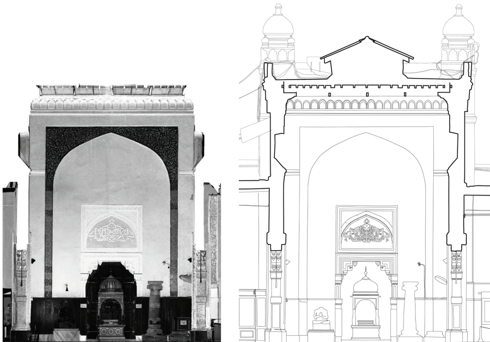
Figure 1.9: Sample drawing prepared from laser scan – ortho-photo (2016) Background Image from Laser scan (left), Sectional Drawing, with internal architectural details (right)
