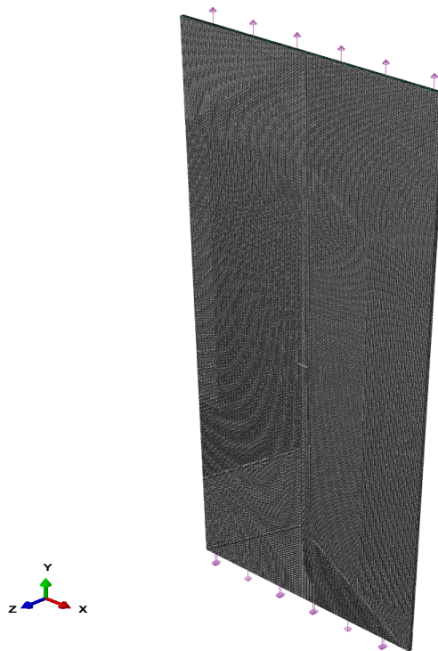
Figure 4.2: FE model of internal cracked specimen.
