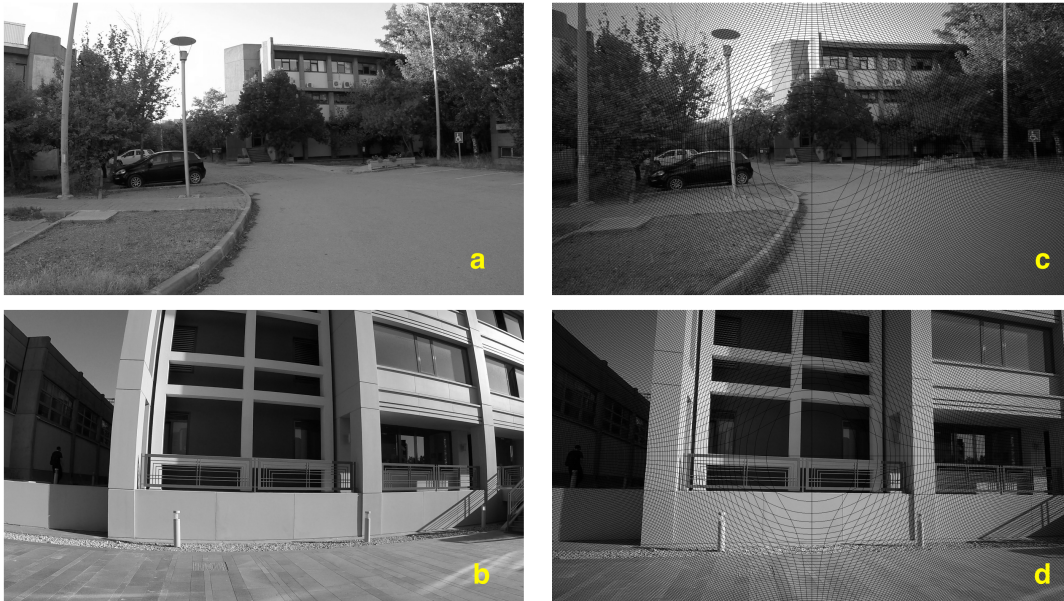
Figure 3.7: In this experiment, stereo image pairs are captured by using GoPro Hero 4 Black camera in two different FOV mode, namely, Medium - \sim 110^\circ and Wide - \sim 140^\circ FOV modes. Images denoted by (a-b) and (c-d) are radially distorted and the undistorted images, respectively, in which removal of radial distortion is done by using our pipeline. Then focal lengths are estimated from these image pairs.
