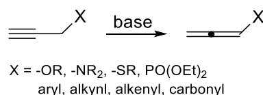
Scheme 9. Isomerization of alkynes to corresponding allenes
