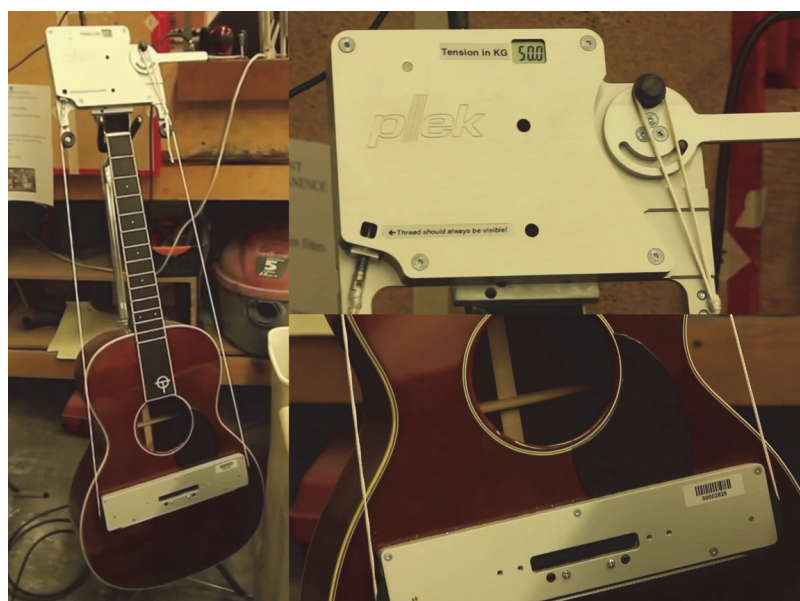
Figure 88 50 kg applied force using exterior STS (String Tension Simulator) Hoover, 2014
