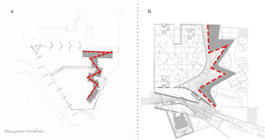
Figure 4.8 Zigzag and its Influence Zone in the Plans of Roofs of Plaza Mayor in Barcelona (a) and Natural Gas Headquarters Building (b)
