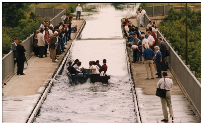
Figure 4.2 Scientists gathered at Heriot-Watt University successfully recreated a solitary wave having smaller dimensions than the one observed by Russell (Hereman, 2013).
