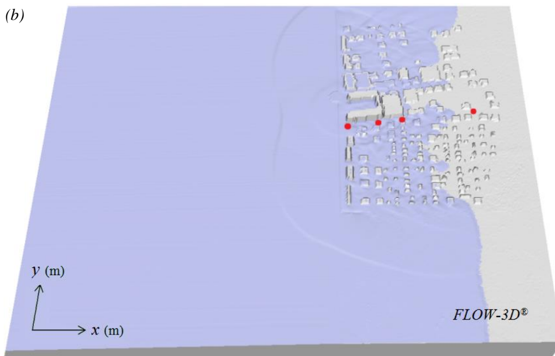
Figure 4.115 Snapshots of (a) NAMI DANCE; (b) FLOW-3D® simulations at time t = 30 sec. The red points correspond to gauges B1 through B9 where the model predictions are compared with the observations.
