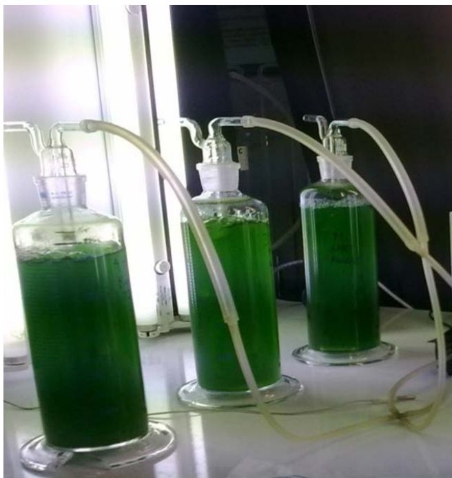
Figure 14 A photo from the experimental setup of the semi-continuous study with primary treated domestic wastewater
