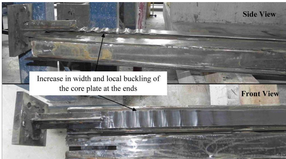
Figure 2.15 Core segment of specimen 2 after testing
