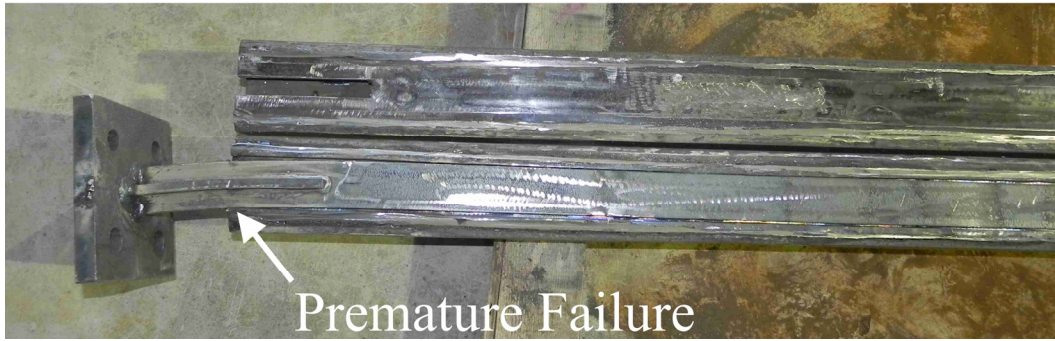
Figure 2.30 Core segment of specimen 9 after testing
