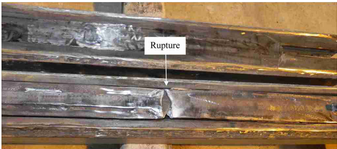
Figure 2.23 Core segment of specimen 6 after testing
