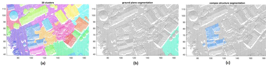
Figure 4.6: Segmentation of Vaihingen point cloud by LSC in 2D view
