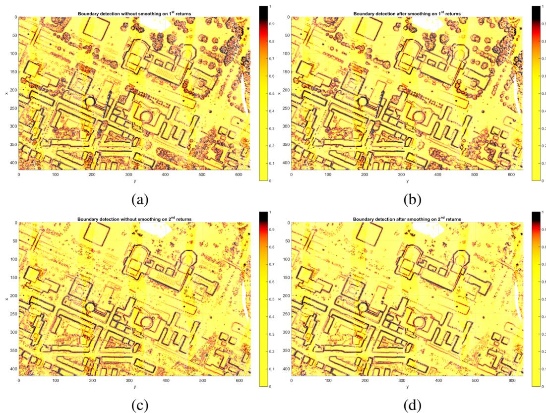
Figure 5.1: Discovered boundaries on 'City Site2'(a) without smoothing on 1<sup>st</sup> returns(b) after smoothing on 1<sup>st</sup> returns (c) without smoothing on 2<sup>nd</sup> returns(d) after smoothing on 2<sup>nd</sup> returns
