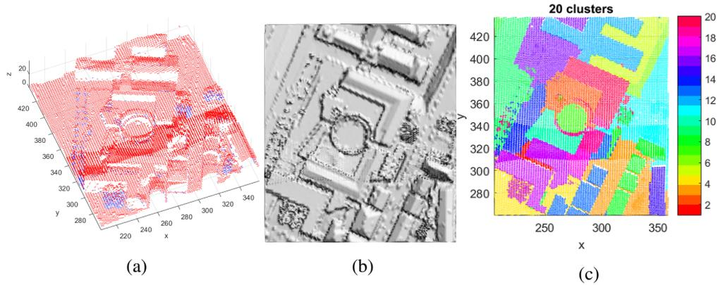
Figure 4.1: (a) ALS data, first returns are shown in red and second returns are blue (b) DEM generated with the given ALS data (c) Segmentation result by the proposed spectral clustering algorithm
