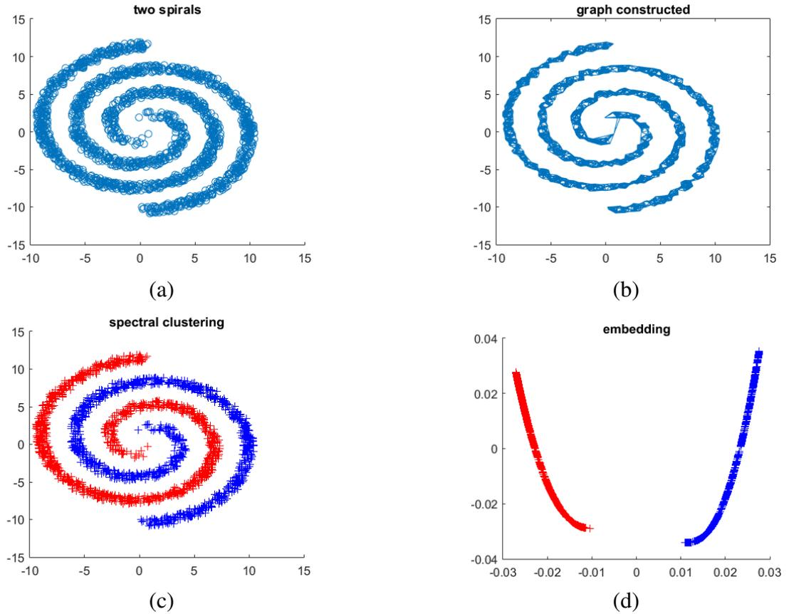
Figure 2.3: (a) Original "Two Spiral" data set (b) Constructed graph topology (c) Clustering on "Two Spiral" (d) 2-dimensional spectral embedding
