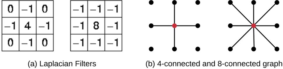
Figure 2.1: Analogy between Laplacian image kernels and Laplacian of graph topologies
