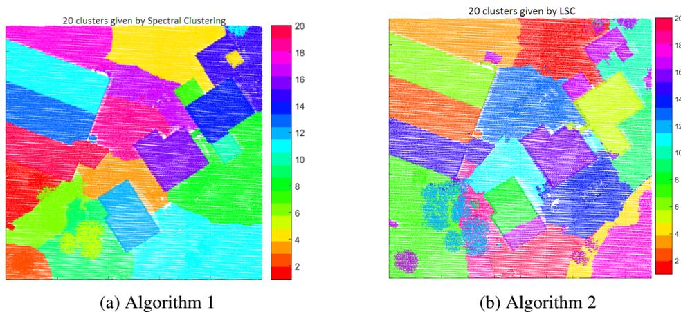
Figure 4.4: Segmentation of "France" point cloud on 2D view
