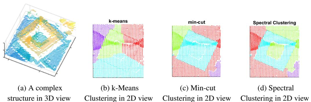
Figure 4.3: Segmentation of a complex building by different clustering methods
