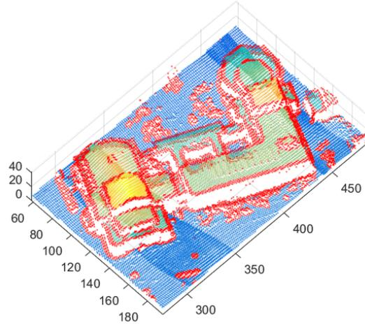
Figure 5.5: Jump edges detected on a multi-layer building (Point cloud is colored with "parula" colormap with respect to elevation values, except the red edge points.)
