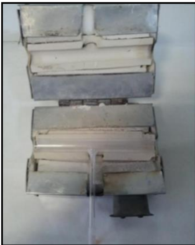
Figure 2.4 Lab-made ceramic electrical heater used to heat QTA to atomization temperature [160] .
