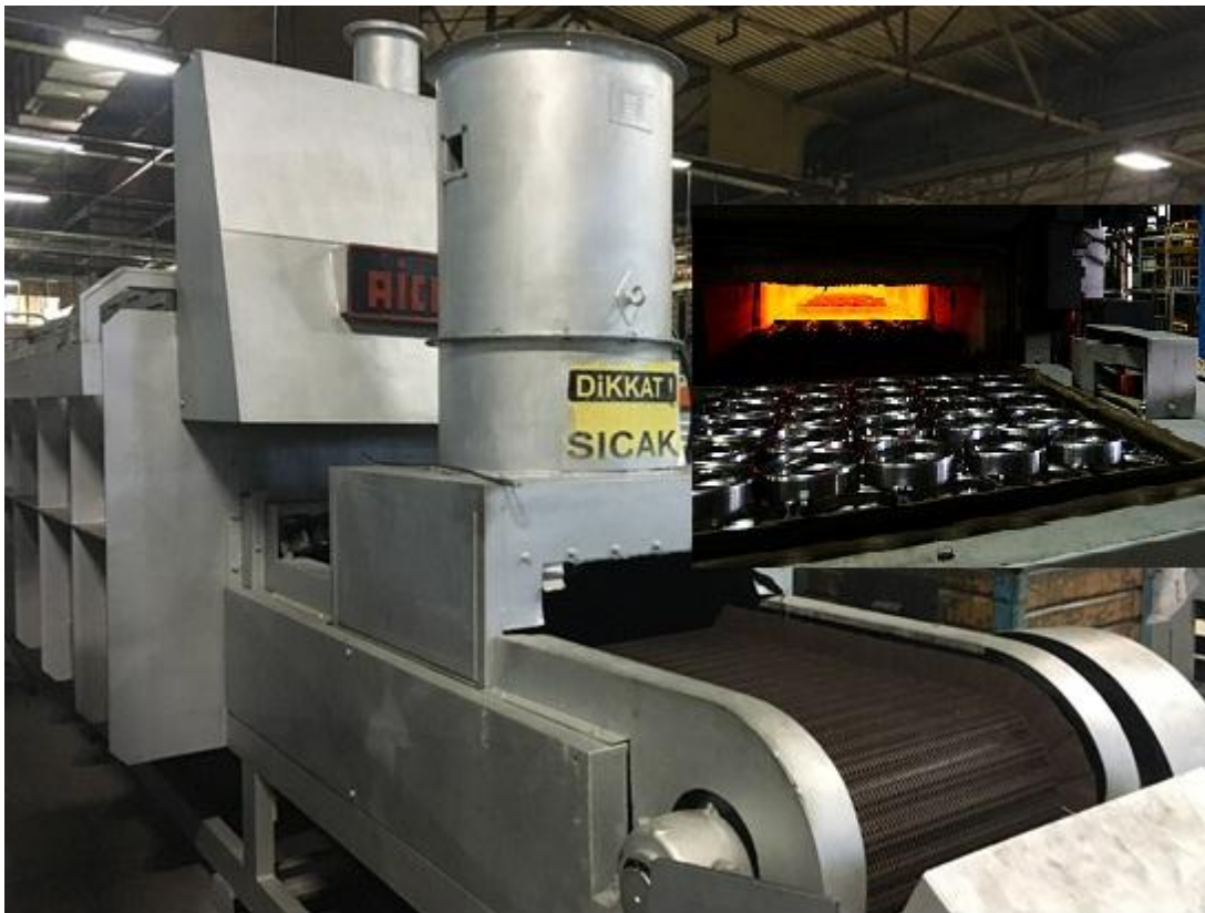
Figure 14 Chamber type tempering furnace
