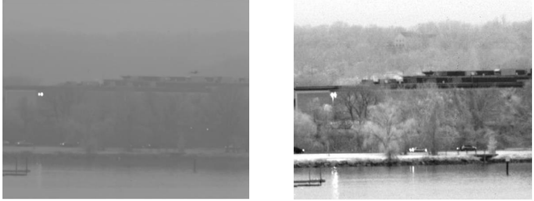
Figure 2.1: Images recorded under hazy conditions by a visible camera (left) and a SWIR camera (right) [12].
