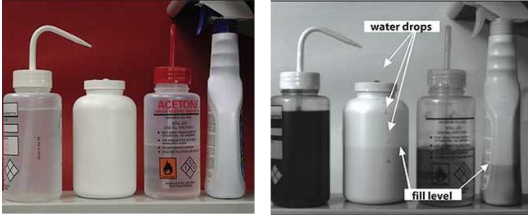
Figure 2.3: The images of opaque and transparent bottles as recorded by a visible camera (left) and a SWIR camera (right) [15].
