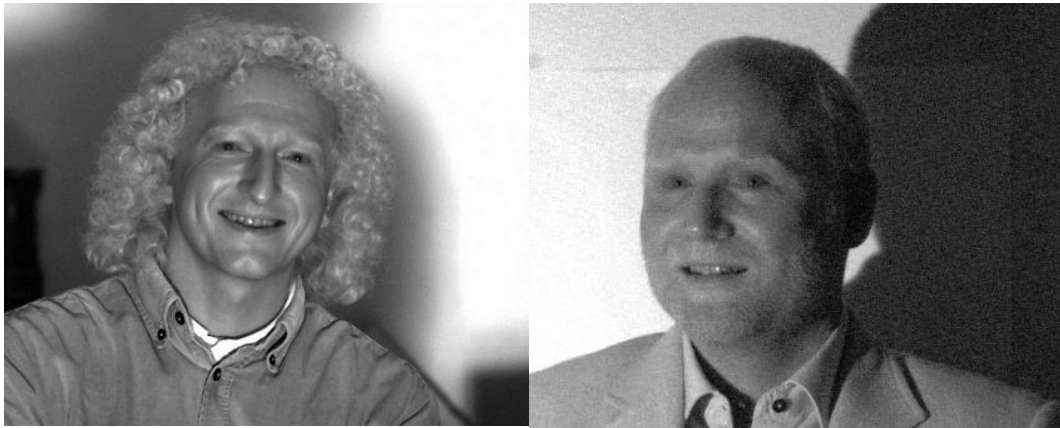
Figure 2.30: An image recorded by a standard InGaAs SWIR camera (left) [57] and by an InGaAs based APDs SWIR camera (right)[58].
