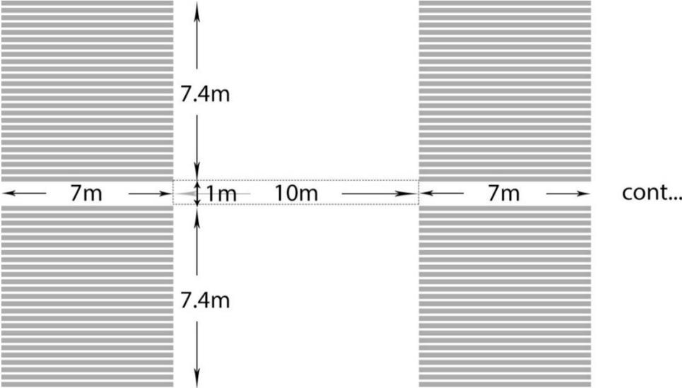
Figure 37: Top views of stack configuration and distances between each of them.
