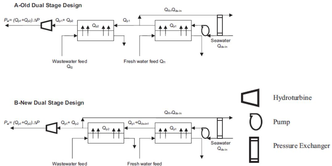
Figure 48 : Comparison of old and new dual stage design for PRO (Altae and Hilal, 2015)
