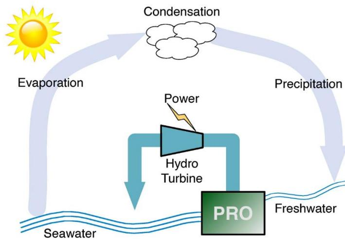
Figure 49: LCA representation of PRO, a renewable source
