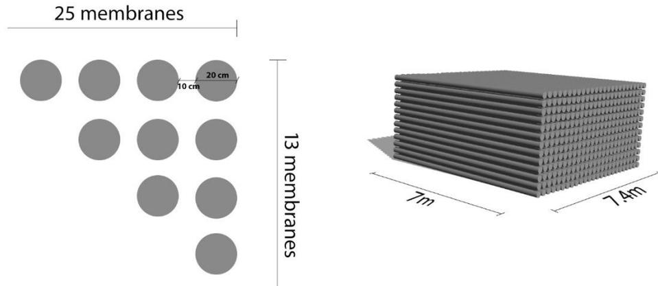
Figure 36: Membrane configuration and dimensions in stack
