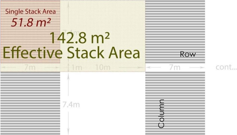
Figure 38: Representation of stack area and effective stack area.
