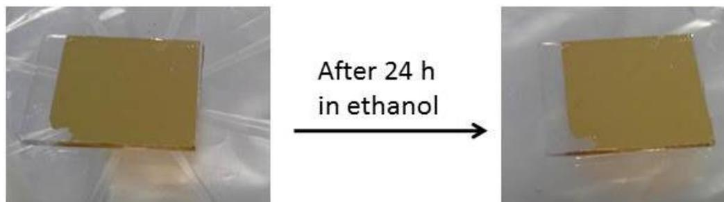
**Figure 45.** Successfully stripped gold by UV-Visible assisted cross linking.
