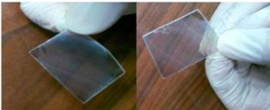
**Figure 77.** Contamination observed on mica substrate upon heating.
