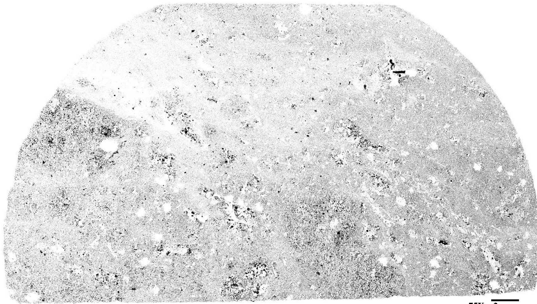
Figure A.1 – C013 Mosaic. Black represents epoxy-filled pores and white represents rock matrix.
