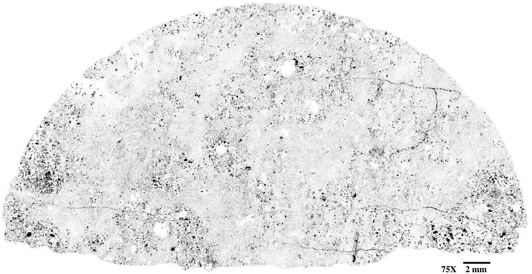
Figure A.2 – C016 Mosaic. Black represents epoxy-filled pores and white represents rock matrix.
