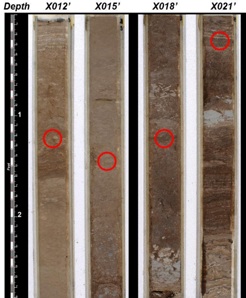
Figure 4.1 – Slabbed core images of carbonate reservoir section in the study well (The plug locations of cores studied, i.e. C013, C016, C019, and C021 are circled in red on the slabbed core images from left to right, respectively).
