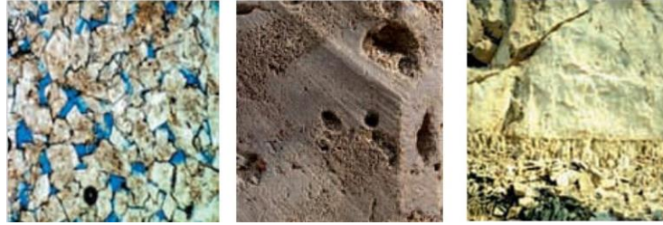
Figure 2.1 – Intergranular pores, vugs and fissures in carbonates from left to right (Schlumberger, 2007).
