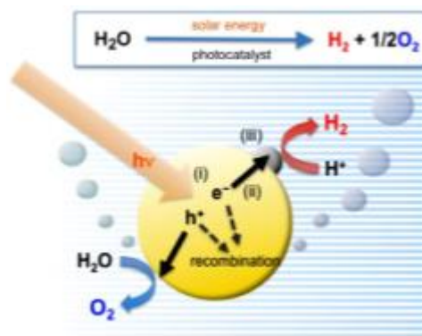
Figure 1.3 Schematic illustration of water spitting over semiconductor photo catalysts [10]
