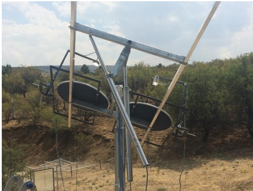
Figure 3.20 Dual axis tracking system with two 70 cm diameter parabolic dishes
