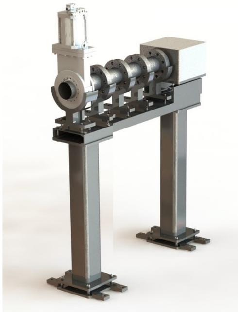
Figure 4.6: The 3D drawing of the energy degradation system for the METU-LEBNA project. It has four titanium foils with  $200 \mu\text{m}$  thickness and three helium sections with the length of 10 cm between them.
