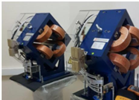
Figure 3.10: Two commercial quadrupole magnets procured from the Scanditronix.
