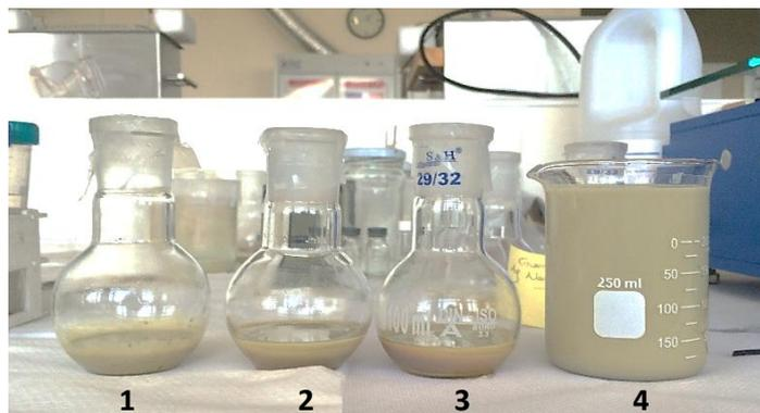
**Figure 4.4** Photos of 1, 2 and 3; Synthesized AgNPs solutions without purification and 4; AgNPs in ethanol.
