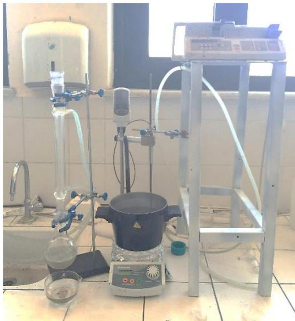
*Figure 4.3 Photo of silver nanoparticle synthesis setup.*
