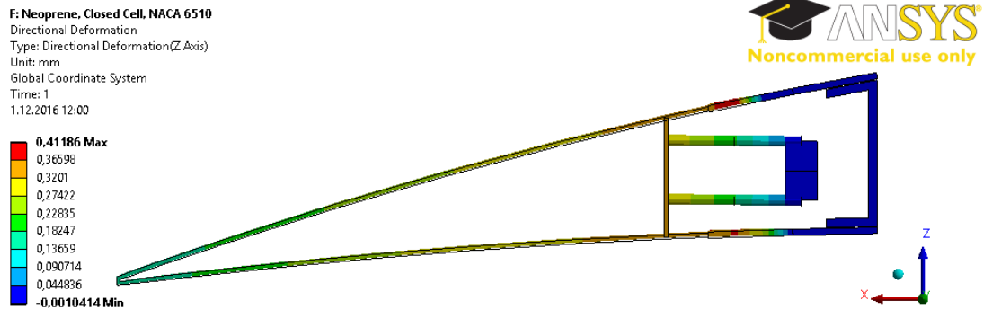
Figure 237: Displacement in z Direction Contour - Maintaining the NACA 6510 Profile under 3g Aerodynamic Loading (Max 0.41 [mm], Closed Cell- Neoprene Rubber Design with 1.0 [mm] composite thickness)
