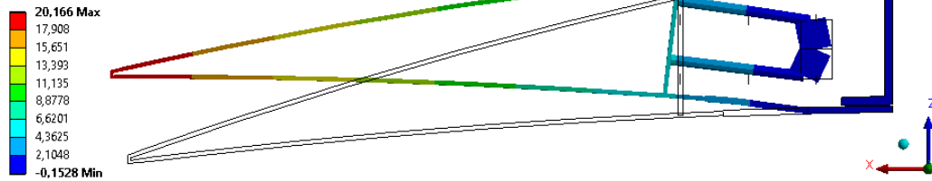
Figure 258: Displacement in z Direction Contour - Morphing from NACA 6510 to NACA 2510 Profile under 2g Aerodynamic Loading (Max 20.17 [mm], Closed Cell-Neoprene Rubber Design with 1.0 [mm] composite thickness)
