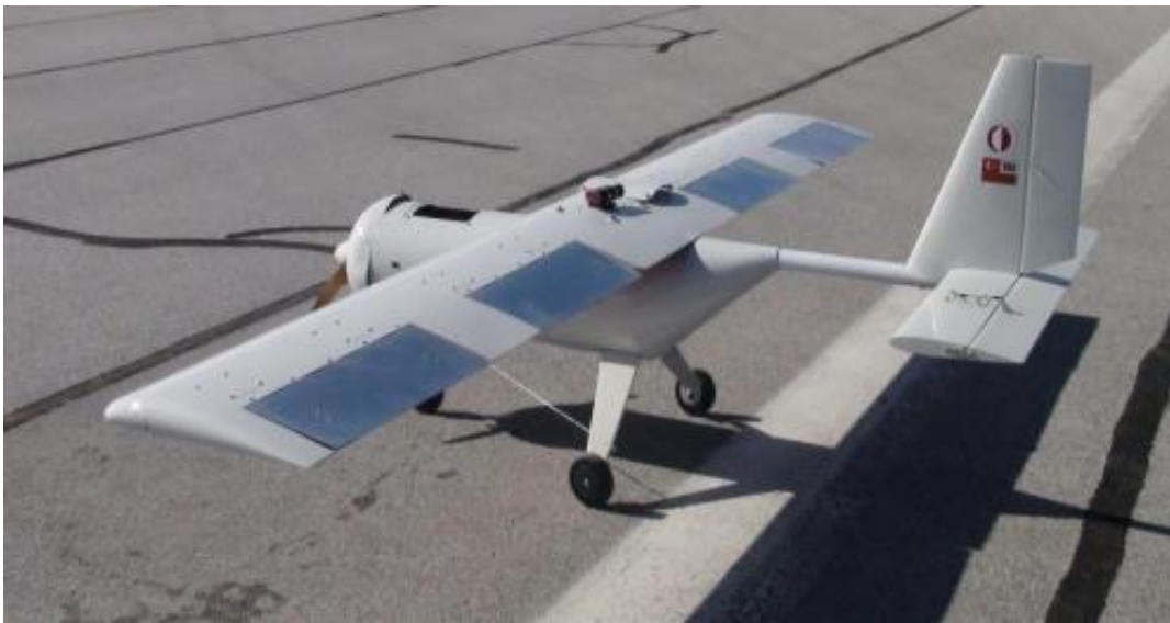
Figure 4: METU’s Indigenously Designed UAV with Hingeless Control Surfaces [16]
