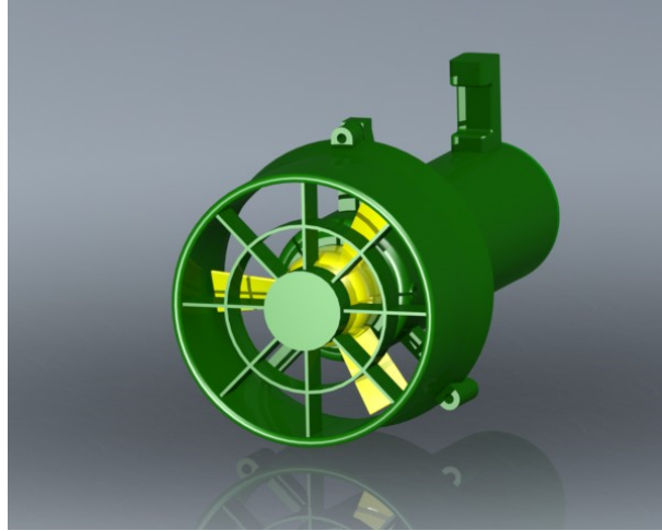
Figure 3.1: Thruster (composed of motor controller-motor-propeller)
