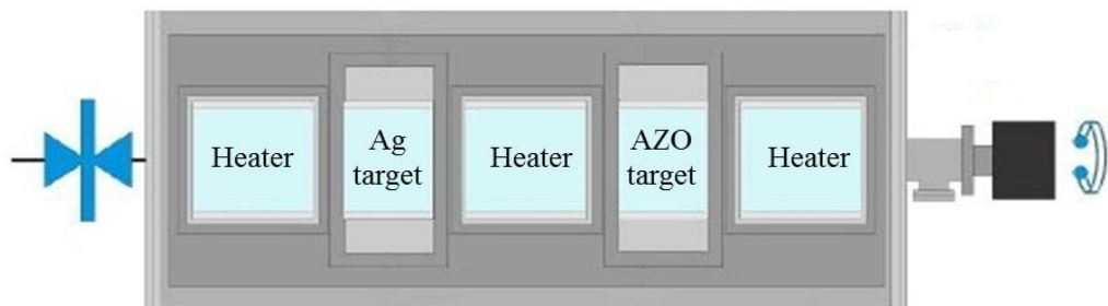
Figure 37: Schematic view of the sputtering chamber
