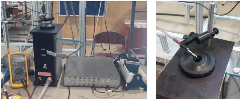
Figure 2. 17: Hot wire calibration setup
