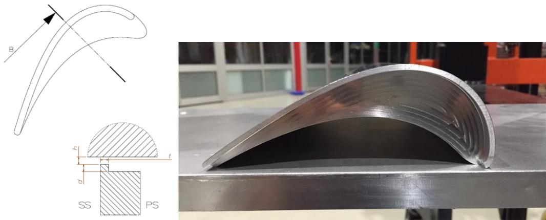
Figure 2. 5: A cross-sectional sketch of HPT bladewith partial squealer tip and manufactured one
