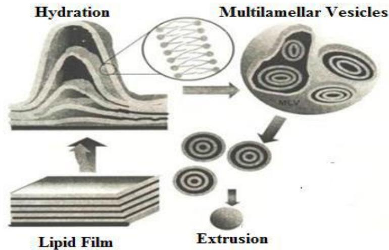
**Figure 1.3.** Illustration of liposome formation with lipid film hydration method (Mansoori et al., 2012)
