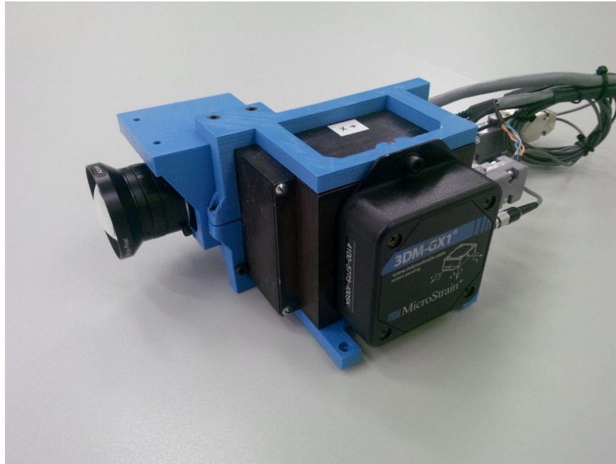
Figure 4.11: The manufactured mounting parts and assembly of the camera, FOG and IMU. The whole structure is designed such that it can also be assembled to the body frame of SensorHex with a couple of auxiliary parts that are also designed and 3D printed.
