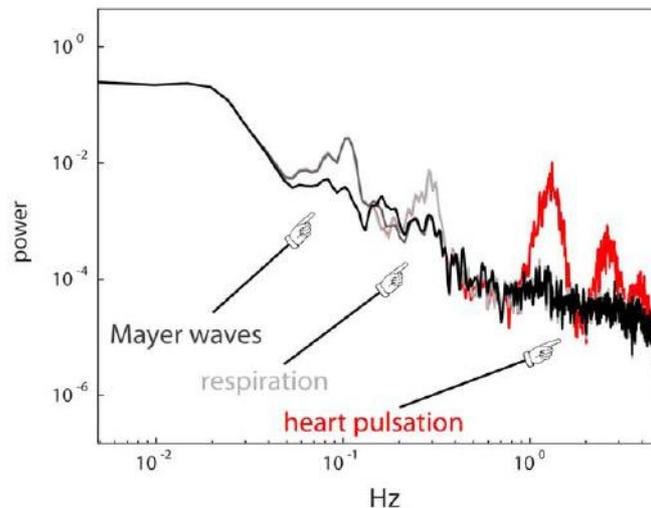
Figure 23. Power spectrum of physiological noises in fNIRS signals.
