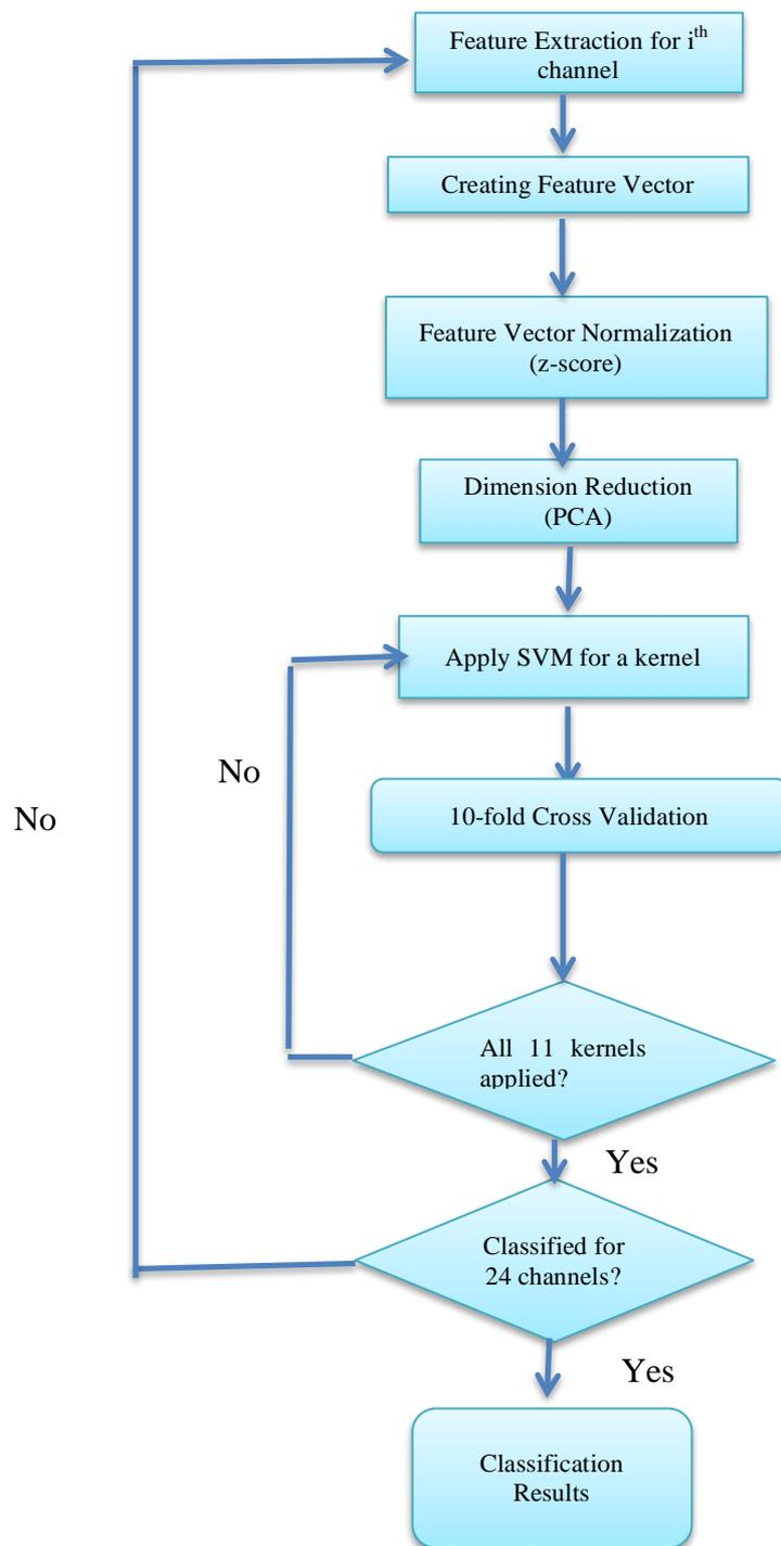
Figure 46. Classification process flow chart for fNIRS data.
